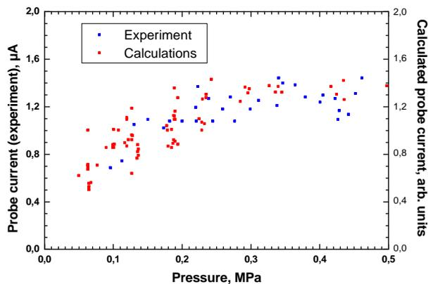
Fig.4. Pressure evolution of probe current: stoichiometric mixture;  $U=-18V$ .
