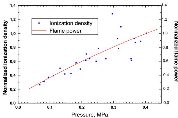
Fig.2. Normalized values of flame ionization density and flame power versus pressure: stoichiometric CH<sub>4</sub> /air mixture.
