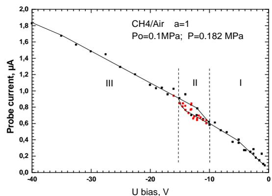
Fig.3 Current-voltage characteristics of ionization probe mounted in combustion chamber wall.
