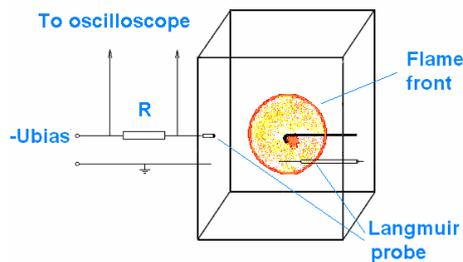
Fig.1. Arrangement of Langmuir probe current measurements.
