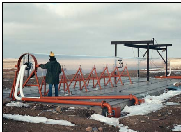
Figure 7 Apparatus used for the study of critical conditions, velocity deficits, and detonation stability
