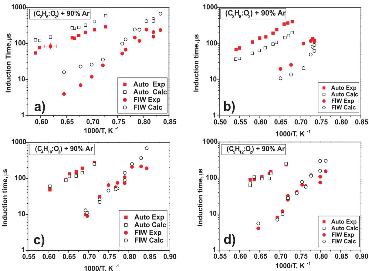
Figure 2: Autoignition (designated as “auto”) and ignition by nanosecond discharge in the form of fast ionization wave (designated as “FIW”) for a)  $\text{C}_2\text{H}_6$ ; b)  $\text{C}_3\text{H}_8$ ; c)  $\text{C}_4\text{H}_{10}$ , and d)  $\text{C}_5\text{H}_{12}$  – containing mixtures. Comparison of experiments and calculations.
