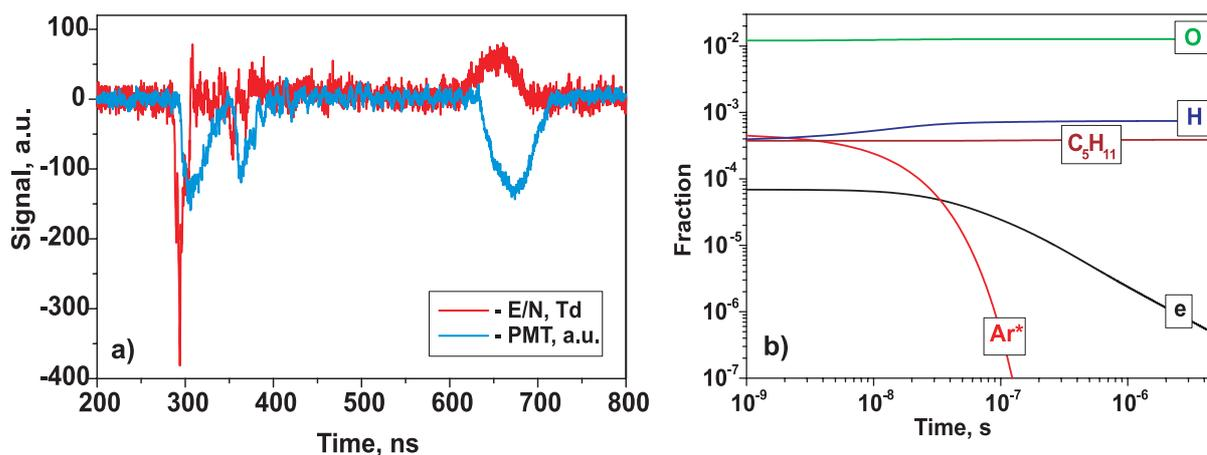
Figure 1: a) – typical temporal behavior of electric field and signal from the photomultiplier.  $\text{CH}_4:\text{O}_2:\text{N}_2:\text{Ar} = 1:4:15:80$  mixture,  $T_5 = 1180$  K,  $P_5 = 0.4$  atm,  $U = -150$  kV; b) – typical calculated densities of active species.  $\text{C}_5\text{H}_{12}:\text{O}_2:\text{Ar} = 1.1:8.9:90$ ,  $T_5 = 1390$  K,  $P_5 = 0.5$  atm,  $U = -110$  kV.
