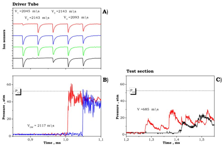
**Figure 3.** Transmission of planar CJ detonation. Pressure (a) and ion current (b) records in the driver tube, pressure (c) records in the main detonation vessel. The initial pressure is 2 atm.
