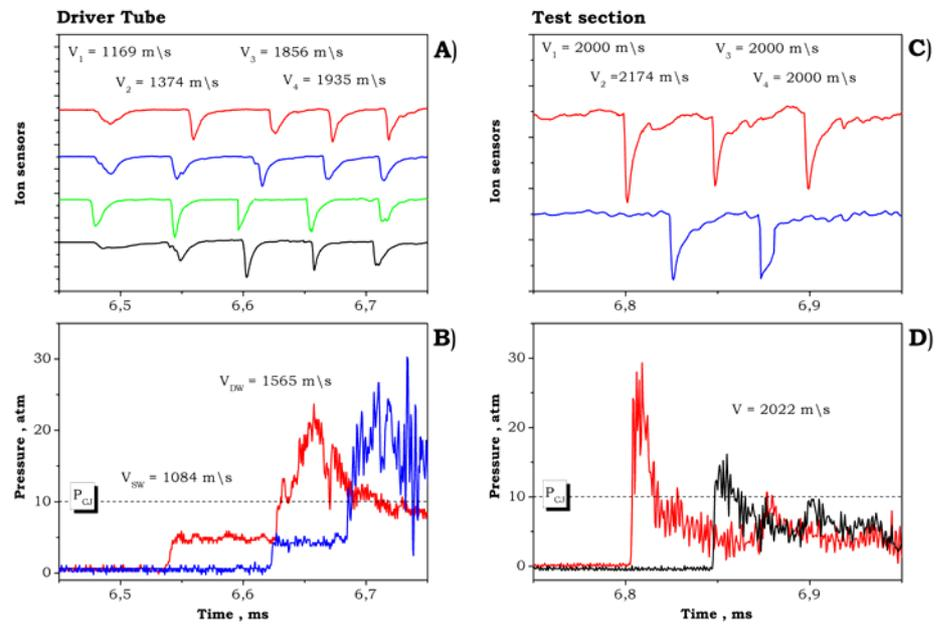
**Figure 2.** Transmission of a shock wave / deflagration complex. Pressure (a) and ion current (b) records in the driver tube, pressure (c) and ion current (d) records in the main detonation vessel. The initial pressure is 0.4 atm.
