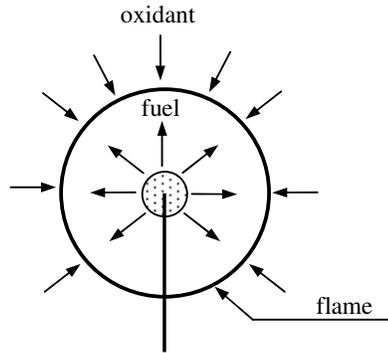
Fig. 1. Schematic representation of the spherical burner.
