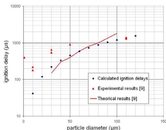
Fig. 6: Estimated ignition delays and comparison with literature
