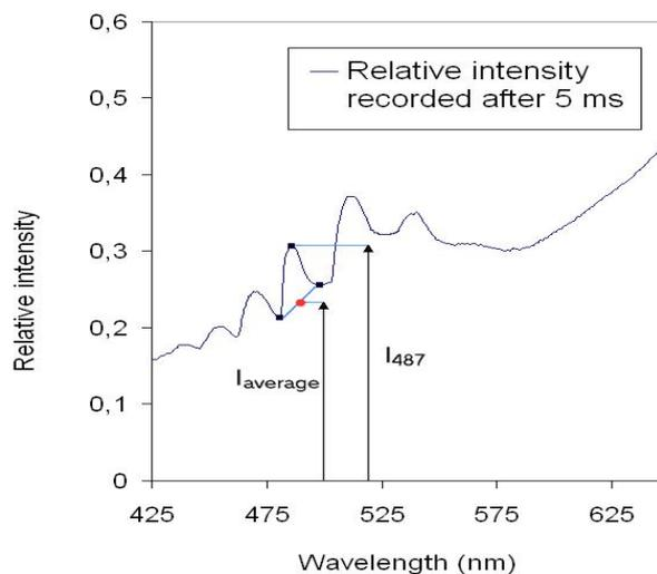
Fig. 2: Definition of  $I_{487}$  and  $I_{\text{average}}$
