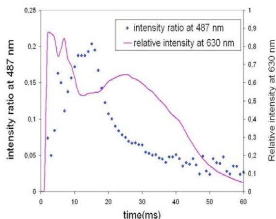
**Fig. 4:** Relative intensity at 630 nm and intensity ratios at 487 nm for 2kg charges containing 5 $\mu\text{m}$  particles.
