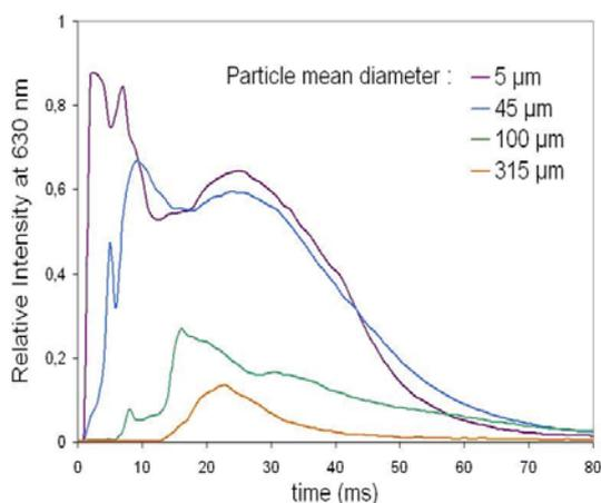
**Fig. 3:** Relative intensity at 630 nm for 2kg aluminized charges
