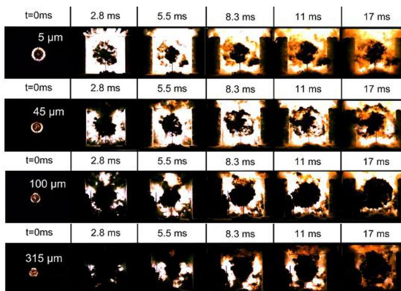
**Fig.1:** Effect of particle diameter on the explosion of 2kg charges in a semi-confined environment.
