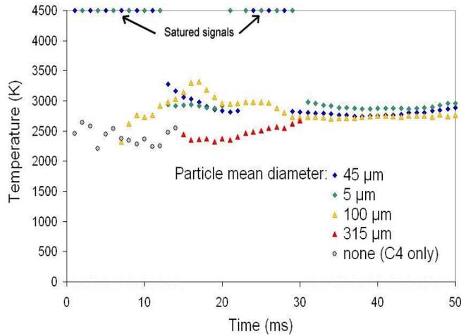
**Fig. 5:** Apparent temperature calculated for different explosive charges containing aluminium particles.
