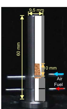
Figure 1. The configuration of miniature combustor
