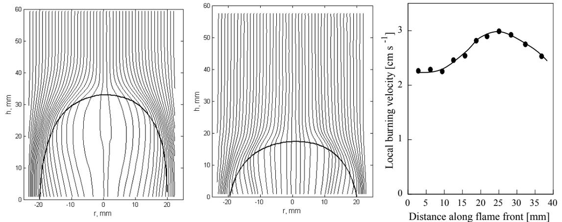
Fig.2. Streamlines recovered from velocity fields shown in Fig.1. a – 5.15% methane flame, b – 5.62% methane flame
