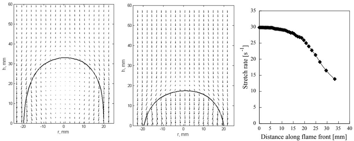
Fig.1. Experimental velocity vector fields in the flame system for 5.15% methane (a)- and 5.62% methane (b) flame in standard tube. Solid line – fitted line for location of maximum divergence of velocity.
