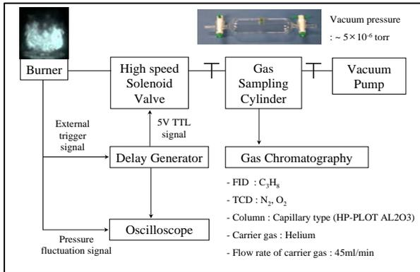
Fig. 3 Schematic diagram of gas sampling system
