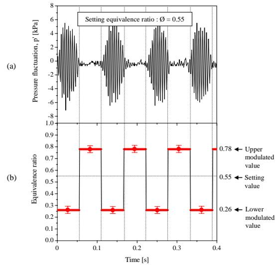
Fig. 4 Modulated equivalence ratio with respect to pressure fluctuation: (a) Pressure fluctuation in the combustion chamber. (b) Modulated equivalence ratio at the fuel supplying holes.
