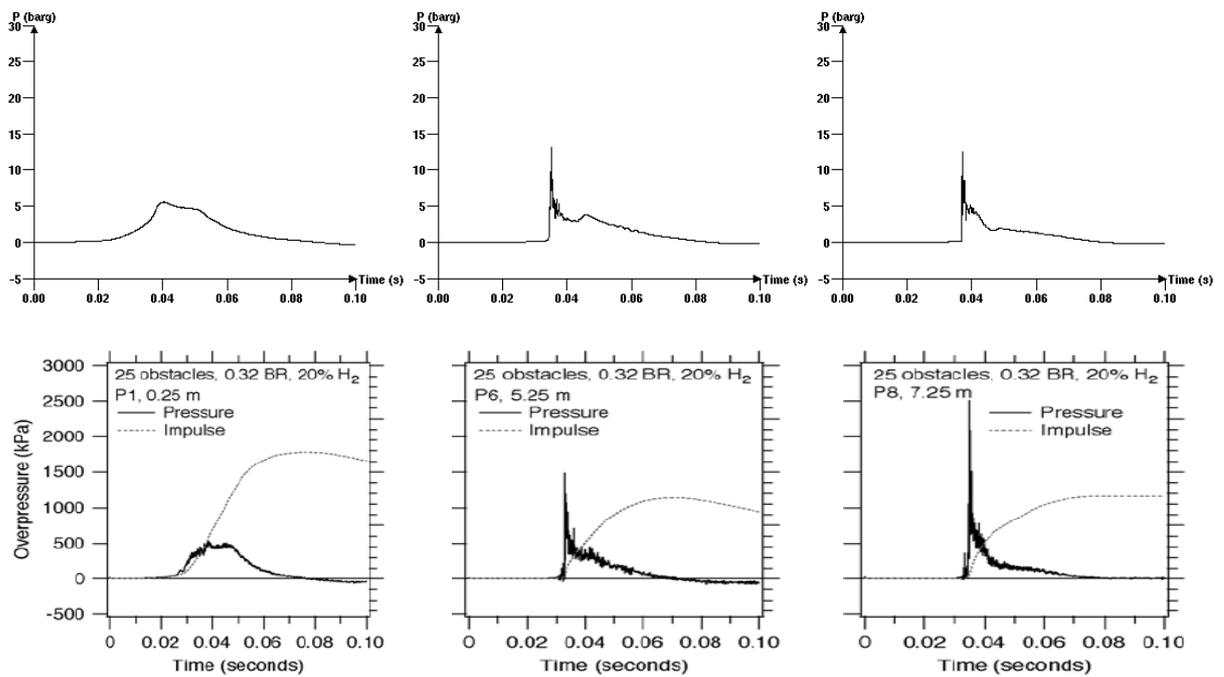
Figure 3. Comparison of simulated pressure traces (top) with experimental results (bottom) at 2 locations
