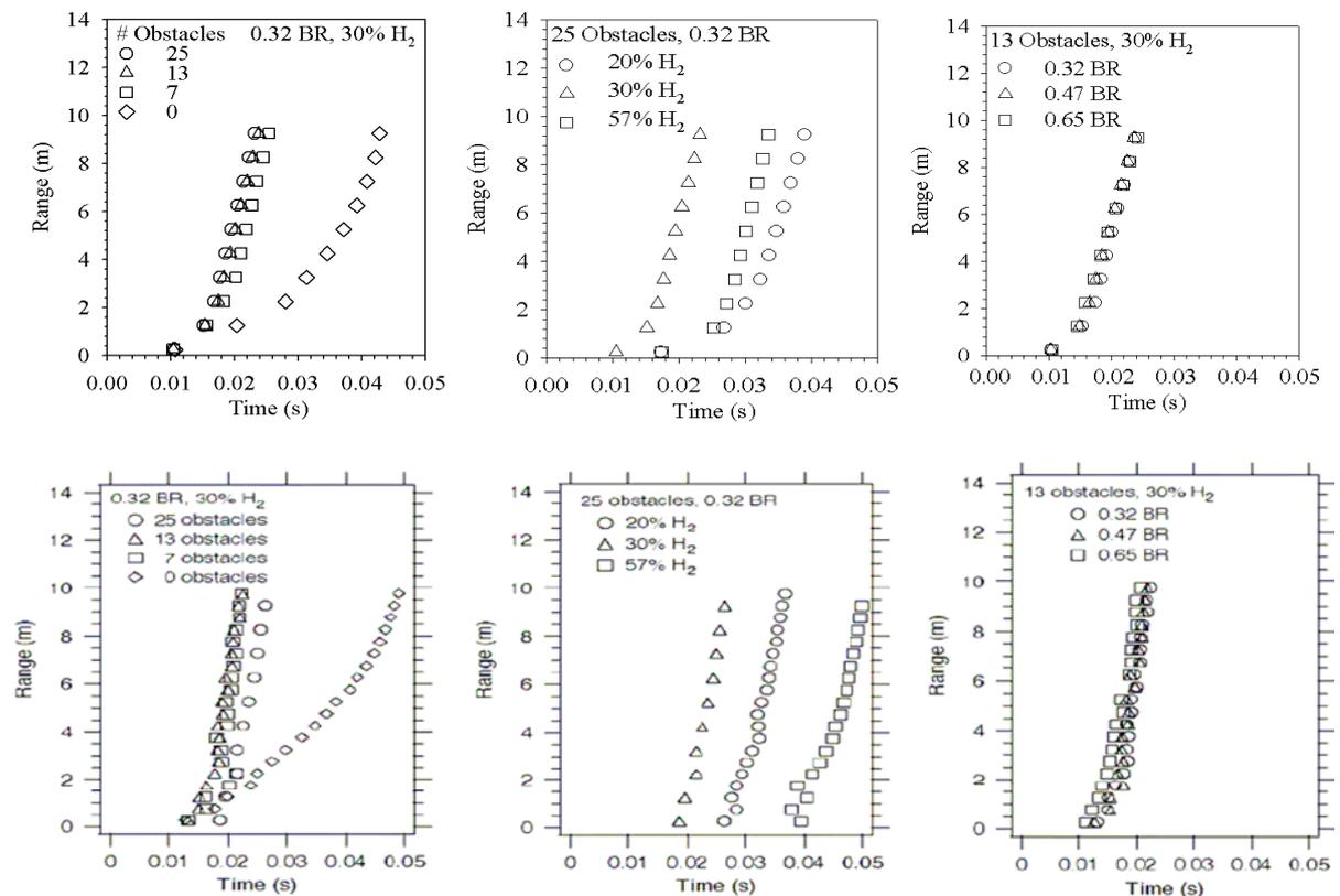
Figure 4. Comparison of simulated flame arrival times (top) with experimental measurements (bottom)
