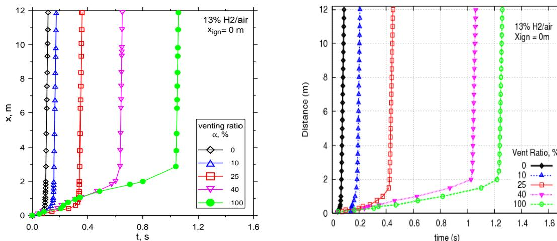
**Figure 1. X-t diagram of the flame propagation from the open end ( $X_{\text{ign}} = 0$  m) and at various vent ratios  $\alpha = 0$ -100%**
