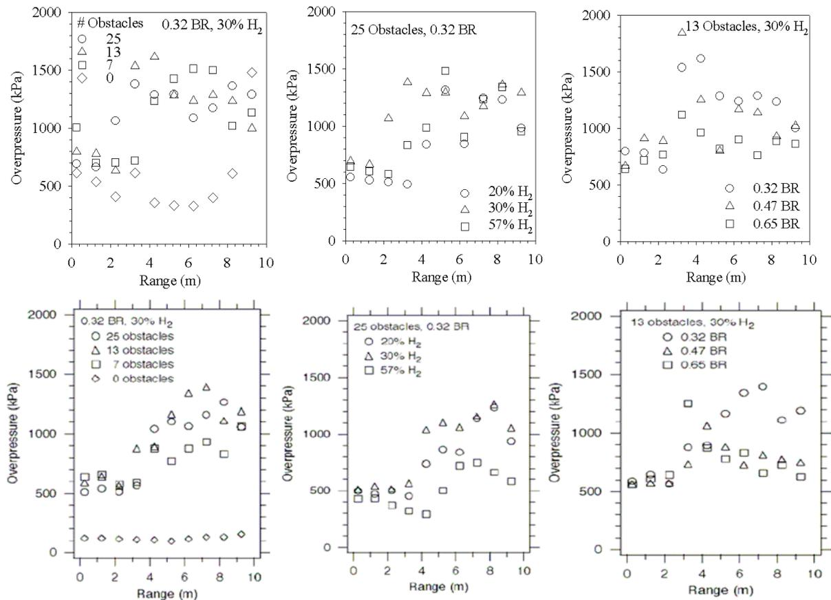
Figure 5. Comparison of simulated overpressures (top) with experimental measurements (bottom)
