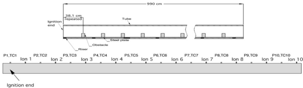
Figure 2. A schematic of the experimental geometry: Tube, obstacle configuration, and sensor details
