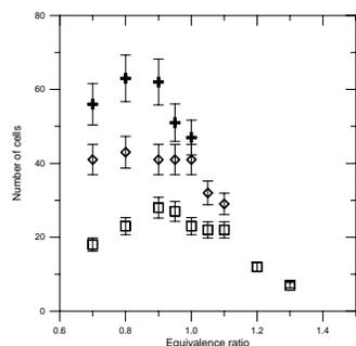
Fig. 6. Number of cells observed in lean (CH<sub>4</sub> + H<sub>2</sub>) + O<sub>2</sub> + CO<sub>2</sub> flames ( $\Phi = 0.8$ ) with hydrogen content  $\alpha = 0.35$ . Crosses: the burner plate temperature = 343 K, diamonds: T = 323 K, squares: T = 303 K.
