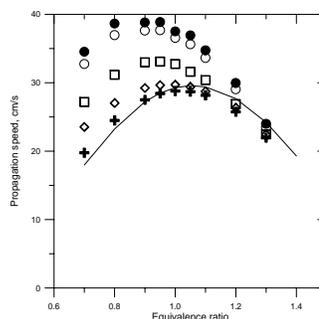
Fig. 3. Propagation speeds in (CH<sub>4</sub> + H<sub>2</sub>) + O<sub>2</sub> + CO<sub>2</sub> flames with hydrogen content  $\alpha = 0.35$ . Crosses: the burner plate temperature = 368 K, diamonds: T = 343 K, squares: T = 323 K, open circles: T = 303 K, solid circles: extrapolated to 298 K, line: adiabatic burning velocity.
