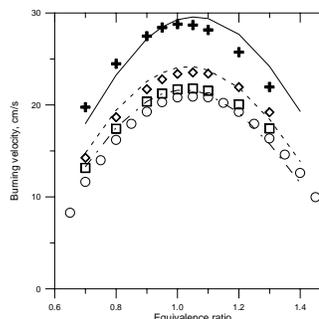
Fig. 4. Laminar burning velocities of (CH<sub>4</sub> + H<sub>2</sub>) + O<sub>2</sub> + CO<sub>2</sub> mixtures. Symbols: experiment, lines: modeling. Crosses and solid line:  $\alpha = 0.35$ ; diamonds and dashed line:  $\alpha = 0.15$ ; circles [1], squares (present work) and dash-dot line:  $\alpha = 0$ .
