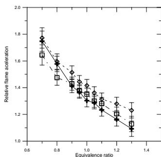
Fig. 5. Ratio of the propagation speed extrapolated to 298 K to the laminar burning velocity in (CH<sub>4</sub> + H<sub>2</sub>) + O<sub>2</sub> + CO<sub>2</sub> flames. Crosses and solid line:  $\alpha = 0.35$ ; diamonds and dashed line:  $\alpha = 0.15$ ; squares and dash-dot line:  $\alpha = 0$ .
