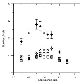
Fig. 7. Number of cells observed in (CH<sub>4</sub> + H<sub>2</sub>) + O<sub>2</sub> + CO<sub>2</sub> mixtures. The burner plate temperature = 303 K. Crosses:  $\alpha = 0.35$ ; diamonds:  $\alpha = 0.15$ ; squares:  $\alpha = 0$ .
