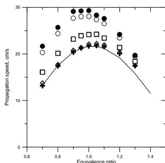
Fig. 1. Propagation speeds in CH<sub>4</sub> + O<sub>2</sub> + CO<sub>2</sub> flames. Crosses: the burner plate temperature = 368 K, diamonds: T = 343 K, squares: T = 323 K, open circles: T = 303 K, solid circles: extrapolated to 298 K, line: adiabatic burning velocity.
