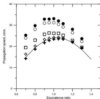
Fig. 2. Propagation speeds in (CH<sub>4</sub> + H<sub>2</sub>) + O<sub>2</sub> + CO<sub>2</sub> flames with hydrogen content  $\alpha = 0.15$ . Crosses: the burner plate temperature = 368 K, diamonds: T = 343 K, squares: T = 323 K, open circles: T = 303 K, solid circles: extrapolated to 298 K, line: adiabatic burning velocity.
