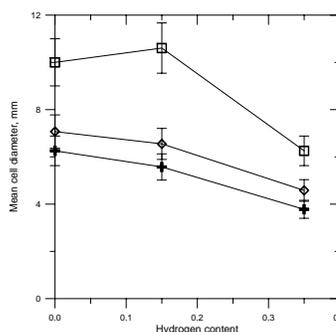
Fig. 8. Mean cell diameter in (CH<sub>4</sub> + H<sub>2</sub>) + O<sub>2</sub> + CO<sub>2</sub> flames as a function of hydrogen content  $\alpha$ . Crosses: the burner plate temperature = 343 K, diamonds: T = 323 K, squares: T = 303 K.
