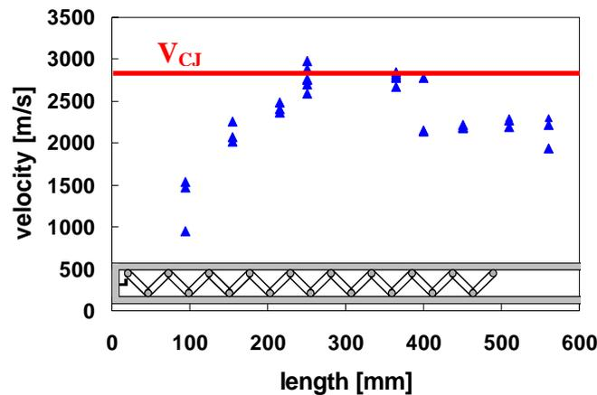
Figure 2 Propagation velocity using the Shchelkin wire for  $2H_2/O_2$  cases.
