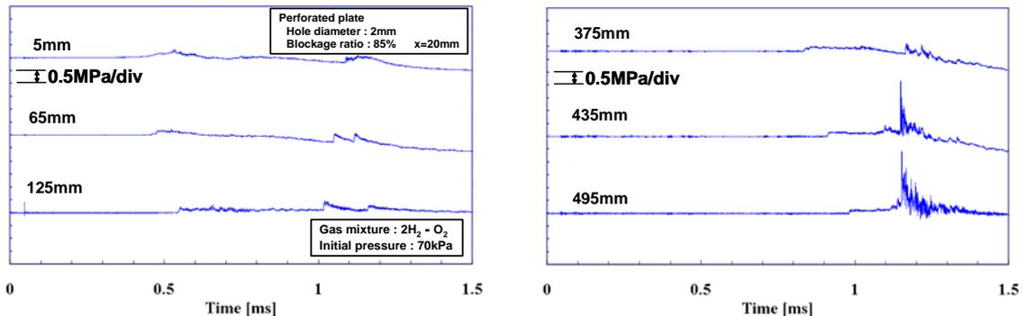
(a) Pressure profiles at 5, 65, and 125 mm from the ignition point using the Shchelkin spiral.
