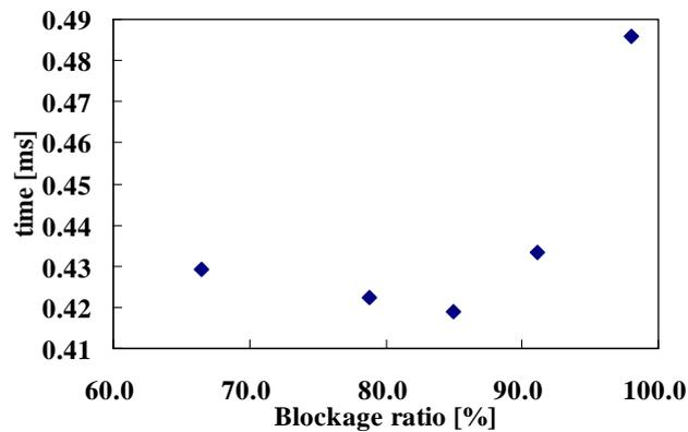
Figure 6 The blockage ratio vs DDT time for the mixture of 2H<sub>2</sub> and O<sub>2</sub>.
