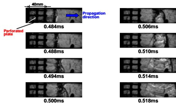
Figure 5 High speed movie photos using two perforated plates.
