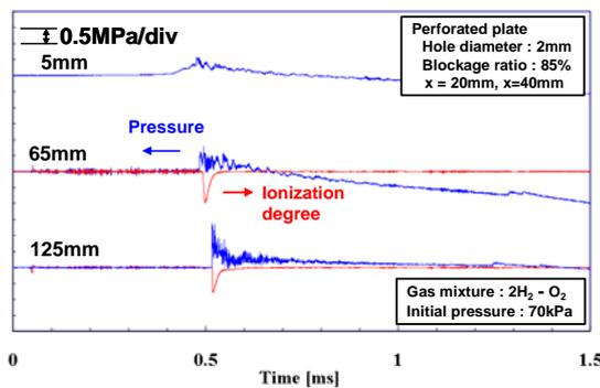
Figure 4 Pressure profiles using two perforated plates
