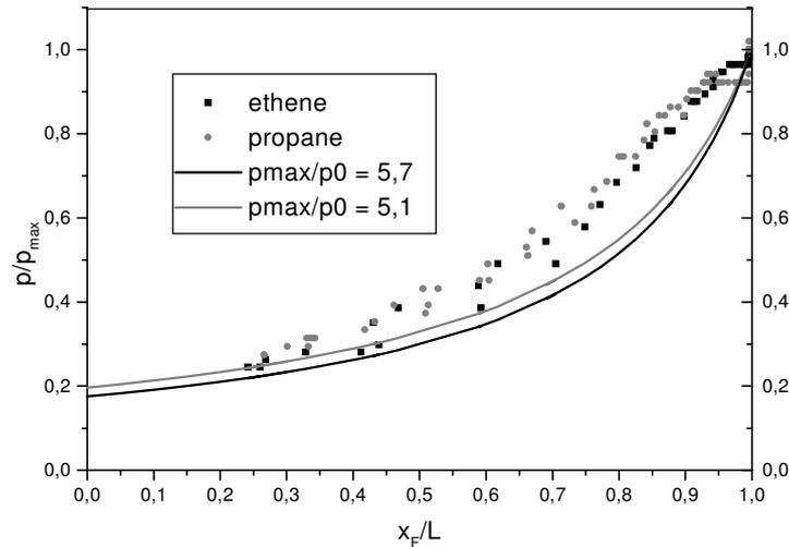
Fig. 3 Explosion pressure  $p$  in dependence on the relative flame front progress  $x_F/L$ . Dots: experimental data,  $L = 2$  m,  $D = 0,69$  mm,  $x_p = 0,5L$ . Lines: Semi-empirical, see text.
