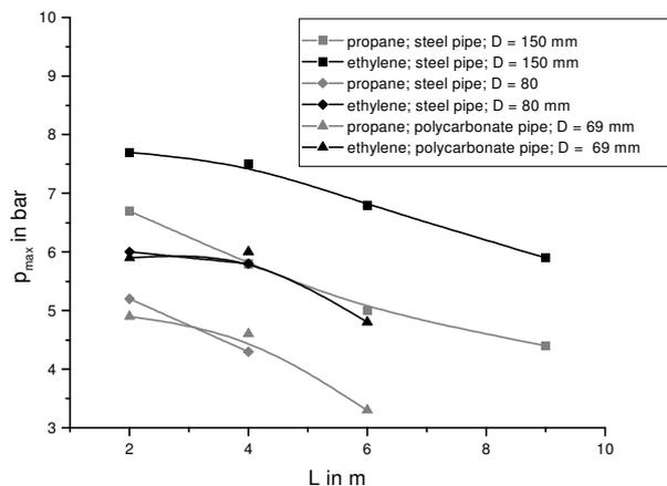
Fig. 2 Maximum explosion pressure in dependence on pipe length  $L$ , pipe diameter  $D$  and pipe material
