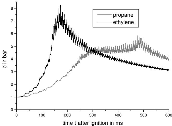
Fig. 1 Explosion pressure in dependence of time  $t$  after ignition. Steel pipe,  $L = 6$  m,  $D = 0,15$  m,  $x_p = 0,5 L$
