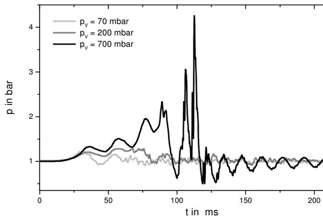
Fig. 4 Effect of venting pressure  $p_v$  on the transient explosion pressure. PVC pipe;  $D = 0,08$  m;  $L = 3,2$  m;  $x_v = 0,5L$ ;  $x_p = 0,8L$ ; propane.
