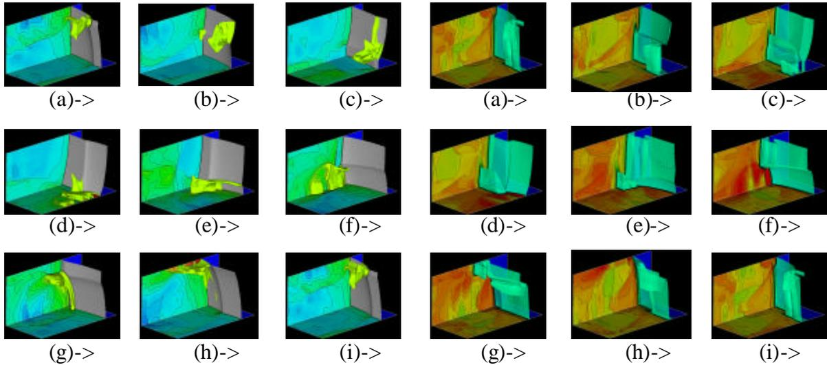
Fig.2 Series of pressure profiles behind spin detonation wave where blue color is 1 atm and red color is 60 atm. The gray is the spin detonation front. Detonation front spins clockwise; (a)->(b)->(c)->(d)->(e)->(f)->(g)->(h)->(i)->(a)->...
