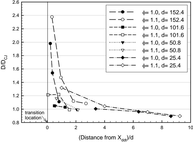
Figure 3 tube diameter effect on the degree of overdriven detonation through DDT process
