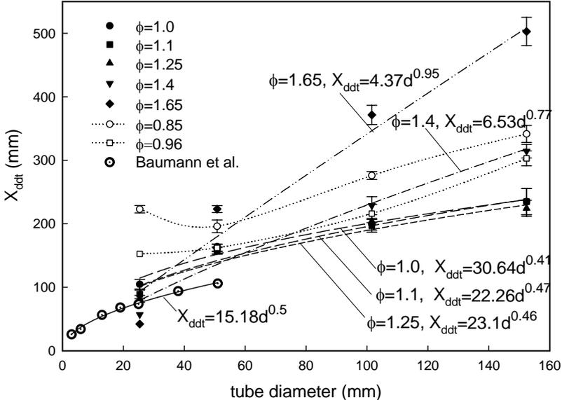
Figure 2 Dependence of  $X_{ddt}$  on tube diameter with fixed  $\phi$
