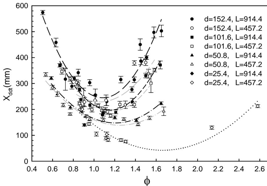
Figure 1 Effect of equivalence ratio on  $X_{ddt}$
