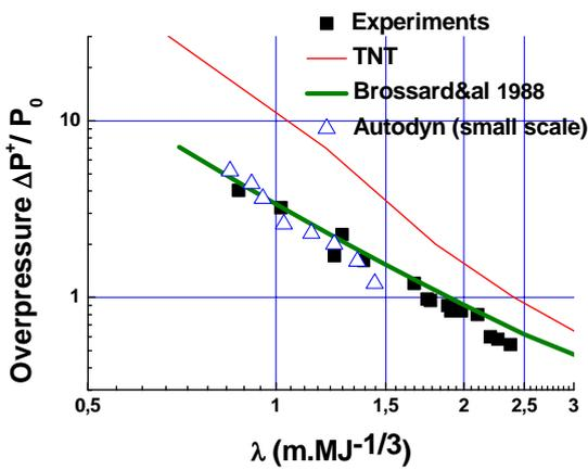
(c) Reflected overpressure,  $\theta_{xy} = 90^\circ$
