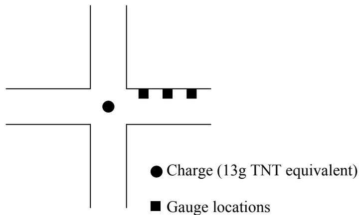
**Figure 5.** Plan of Cross-Roads Small Scale Experiment Geometry (Fairlie & al 2000)
