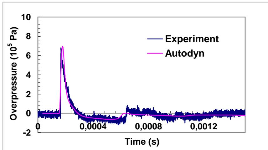
**Figure 8.** Reflected pressure wave profile: experimental and numerical models (gauge located at the center of the face,  $R_0 = 0.06 m$ ,  $r = 0.15 m$ , small scale)
