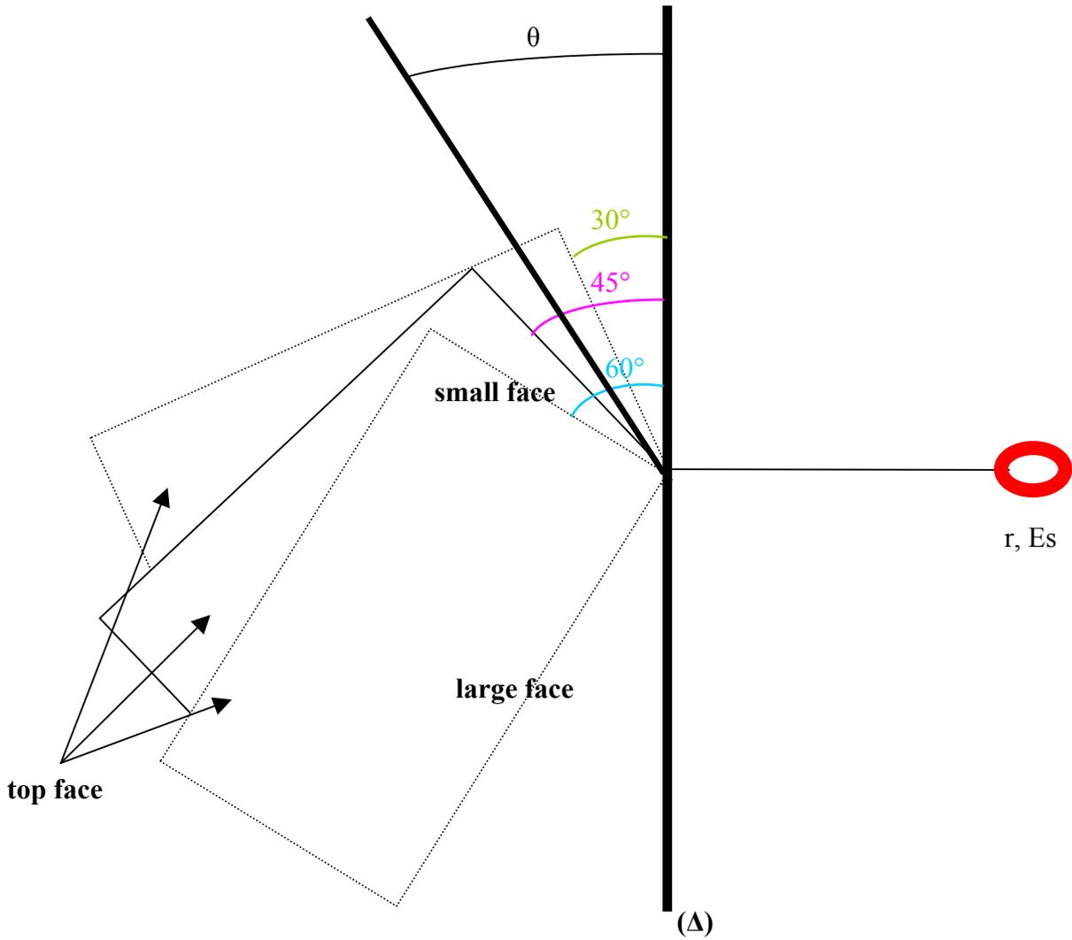
**Figure 3.** Top view of the parallelepipedic structure: position of the explosive charge defined with the angle  $\theta$ .
