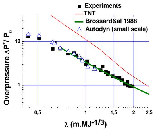
**(b)** Reflected overpressure,  $\theta_{xy} = 0^\circ$
