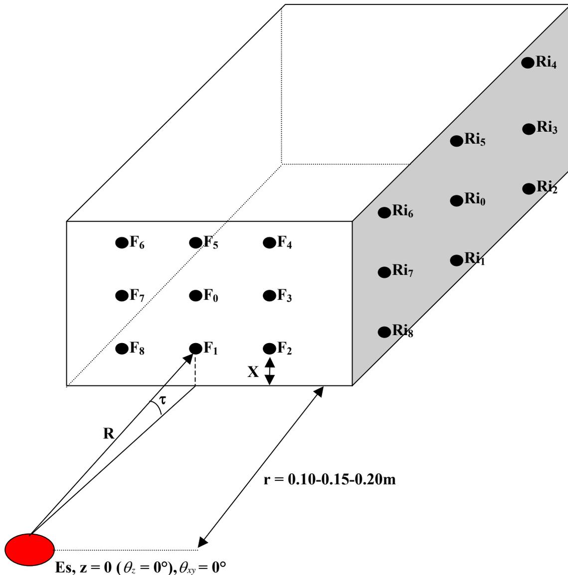
**Figure 6.** Location of gauges on the parallelepipedic structure,  $\theta_{xy} = 0^\circ$  et  $\theta_z = 0^\circ$  ( $z=0$ )
