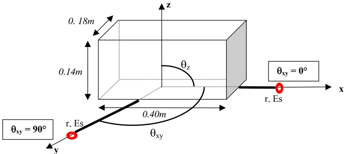
**Figure 2.** The experimental setup: the parallelepipedic structure and the different positions of the explosion source Es. ( $r = 0.10 - 0.15 - 0.20$  cm,  $\theta_z = 0^\circ$ ).
