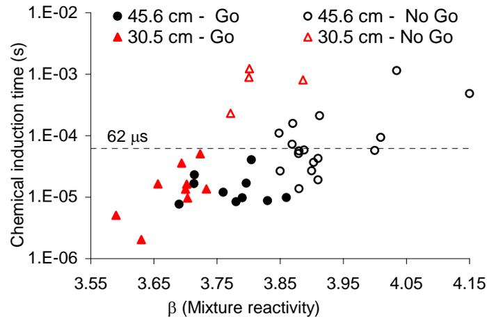
Figure 4. Calculated induction time based on reflected shock state for 0.87 BR reflector orifice plate, expansion time shown as dashed line
