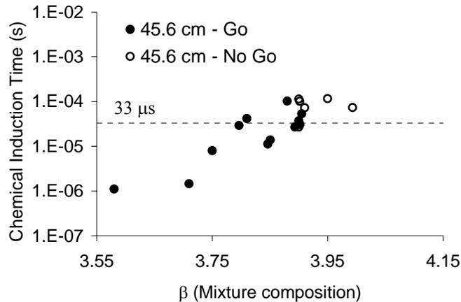
Figure 5. Calculated induction time based on reflected shock state for 0.6 BR reflector orifice plate, expansion time shown as dashed line
