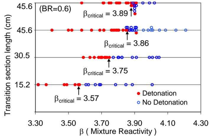
Figure 3. Critical mixtures for detonation initiation for BR= 0.87 reflector except where noted
