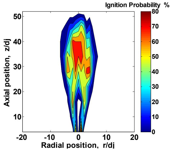
**Figure 1.** Ignition probability of a diluted methane jet flame (70%CH<sub>4</sub>, 30%air)  $U_j = 12.5$  m/s. Spark: 400  $\mu$ s, 100 mJ, 1 mm electrode, 1 mm gap.
