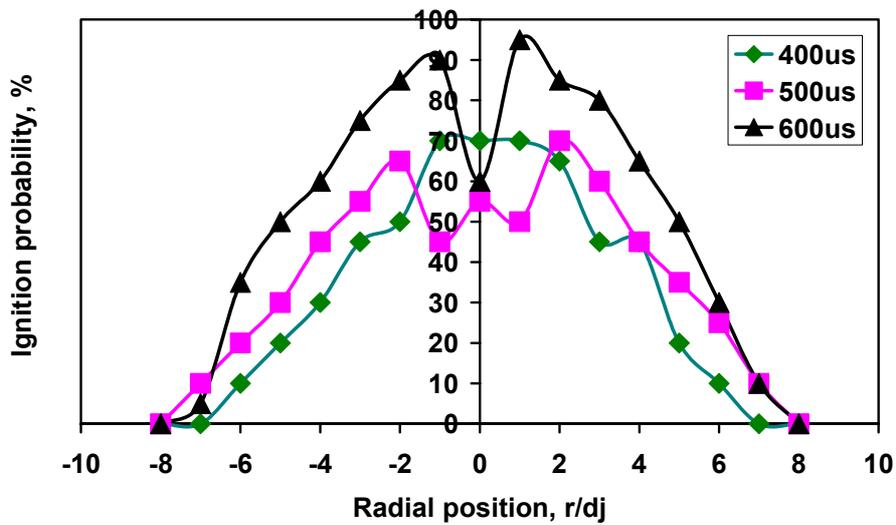
**Figure 2.** Radial profile of the ignition probability as a function of spark duration.  $z/dj = 40$ ,  $U_j = 12.5$  m/s. Spark: 100 mJ, 1 mm electrode, 1 mm gap.
