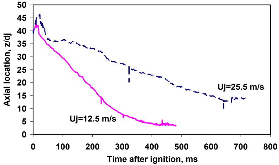
**Figure 3.** Flame position as a function of time for a mixture 70%CH<sub>4</sub> and 30%air (by vol.). Spark: 400  $\mu$ s, 100 mJ, 1 mm electrode, 1 mm gap.
