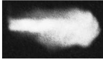
Figure 12. Form of air-plasma jet at the weak electrical field
