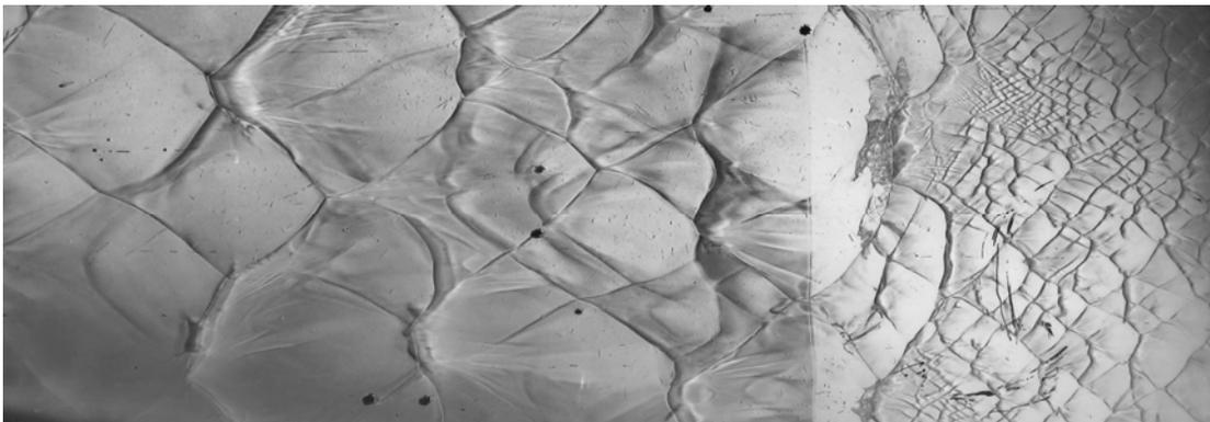
**Figure 4.** Smoked foil records showing the evolution of cellular pattern of the detonation after collision with a shock wave
