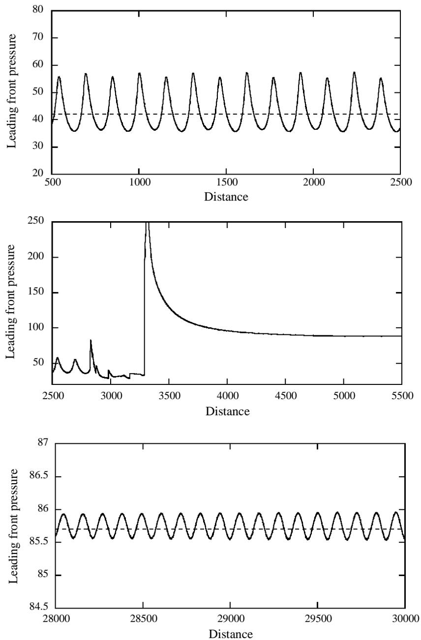
**Figure 2.** Leading front pressure versus position of the unstable detonation colliding with an incident shock of different strength  $M_s$ ; (top) before collision; (middle) early development subsequent to the collision; and (bottom) after long-time evolution subsequent to the collision. Dashed Line represents the Von Neumann pressure based on the CJ solution from steady-state analysis for both incident and transmitted detonations.
