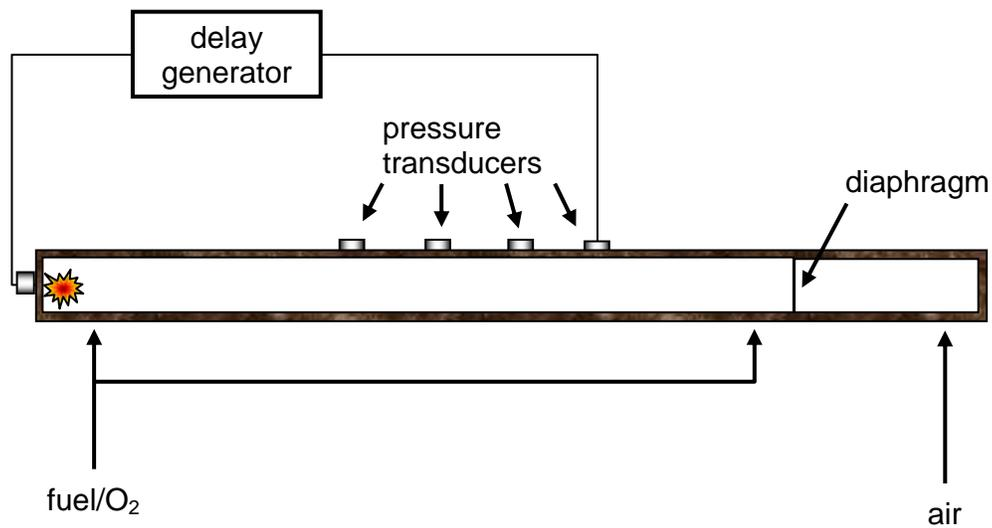
**Figure 3.** Schematic of experimental apparatus
