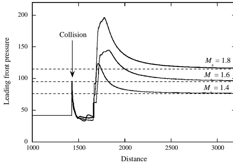
**Figure 1.** Leading front pressure versus position of the detonation colliding with an incident shock of different strength  $M_s$ . Dashed Line represents the Von Neumann pressure based on the CJ solution from steady-state analysis for transmitted detonation.
