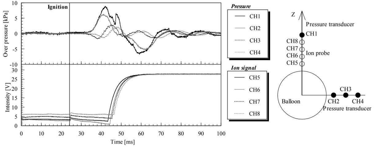
Figure 2 Time-series data of high-speed images, pressure, and ion current signals. (experimental condition:  $\phi=1.8$ ,  $d=150\text{cm}$ ,  $h=40\text{cm}$ , ignition: after break of balloon)
