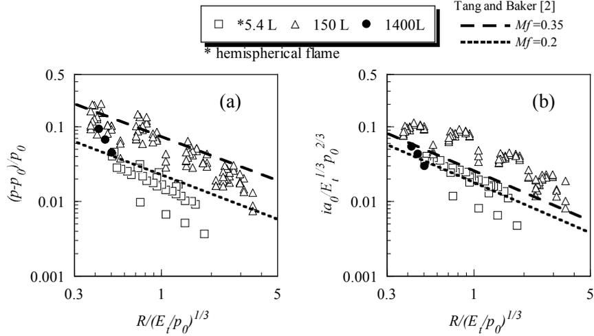
Figure 3 Sachs's scaling law. (a) Normalized peak over pressure versus normalized distance, (b) Normalized positive impulse versus normalized distance.
