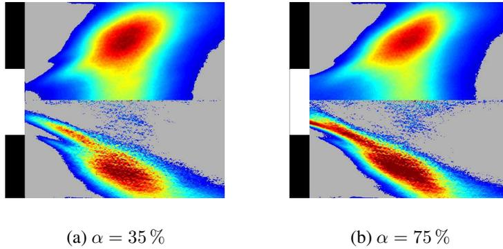
Figure 4: Influence of the staging parameter on the flame structure ( $\text{OH}^*$  emission) -  $Q_{\text{air}} = 40 \text{ Nm}^3 \cdot \text{h}^{-1}$ ,  $\phi = 0.82$ . On top: mean images - On bottom: Abel transform.
