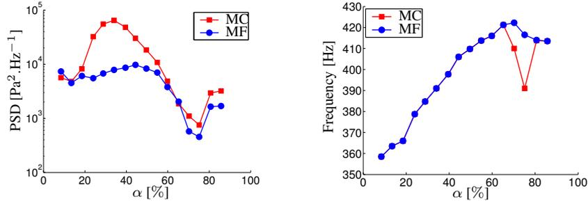
Figure 3: Spectral analysis of the burner of both microphones -  $Q_{\text{air}} = 40 \text{ Nm}^3 \cdot \text{h}^{-1}$  -  $\phi = 0.82$ .
