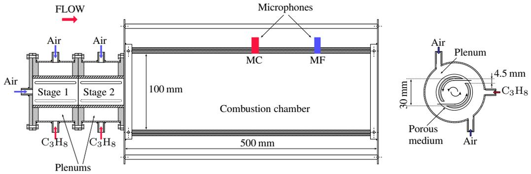
Figure 1: *Schematic of experimental device - Left side: global set-up - Right side: detailed transverse view of gas distribution in one stage.*
