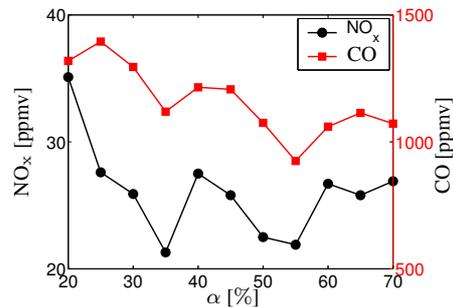
Figure 2: *Pollutant emissions ( $\text{NO}_x$  and CO concentrations) of the burner measured in the middle of the combustion chamber*
