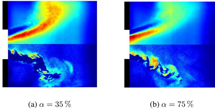
Figure 5: *OH PLIF in a longitudinal view -  $Q_{\text{air}} = 40 \text{ Nm}^3 \cdot \text{h}^{-1}$ ,  $\phi = 0.82$ . On top: mean image - On bottom: instantaneous (25 ns) shot.*
