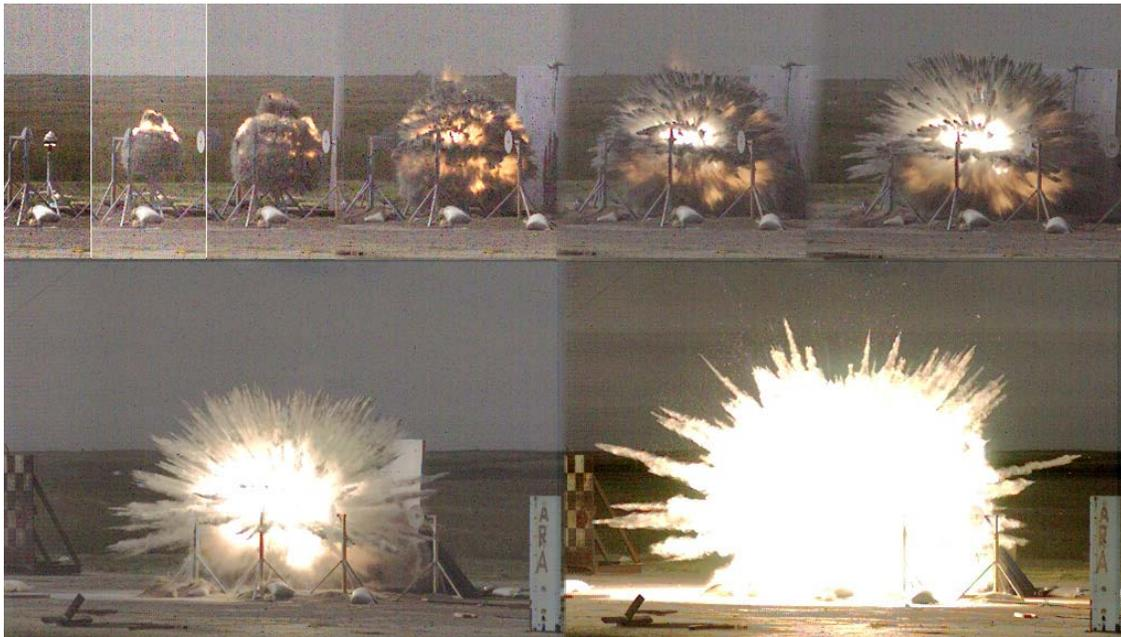
Fig. 3 Development of particle jets during the dispersal of  $10 \mu\text{m}$  aluminum powder from a 1-liter charge. Times of photographs are 0.1, 0.5, 1, 2, 3, 4, 6, and 10 ms, respectively.
