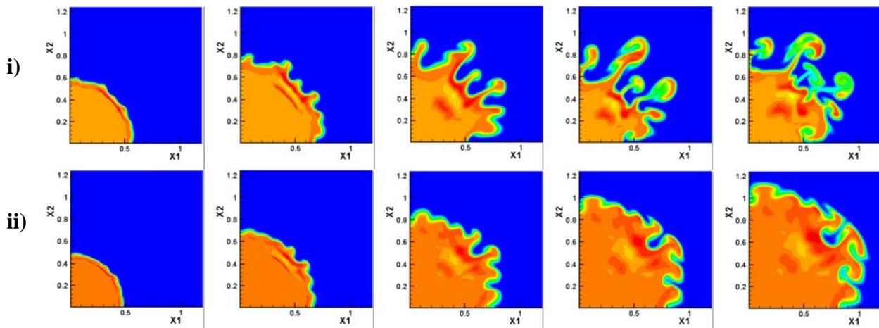
Fig. 5 Computation of the development of instabilities on the interface of a high-pressure cylindrical gas volume expanding (i) after an instantaneous energy release, and (ii) with 50% of the total energy released immediately and the remainder of the energy released within the products over several milliseconds. Times for the pictures in both cases are 0.25, 0.50, 1, 2, and 3 ms, respectively.
