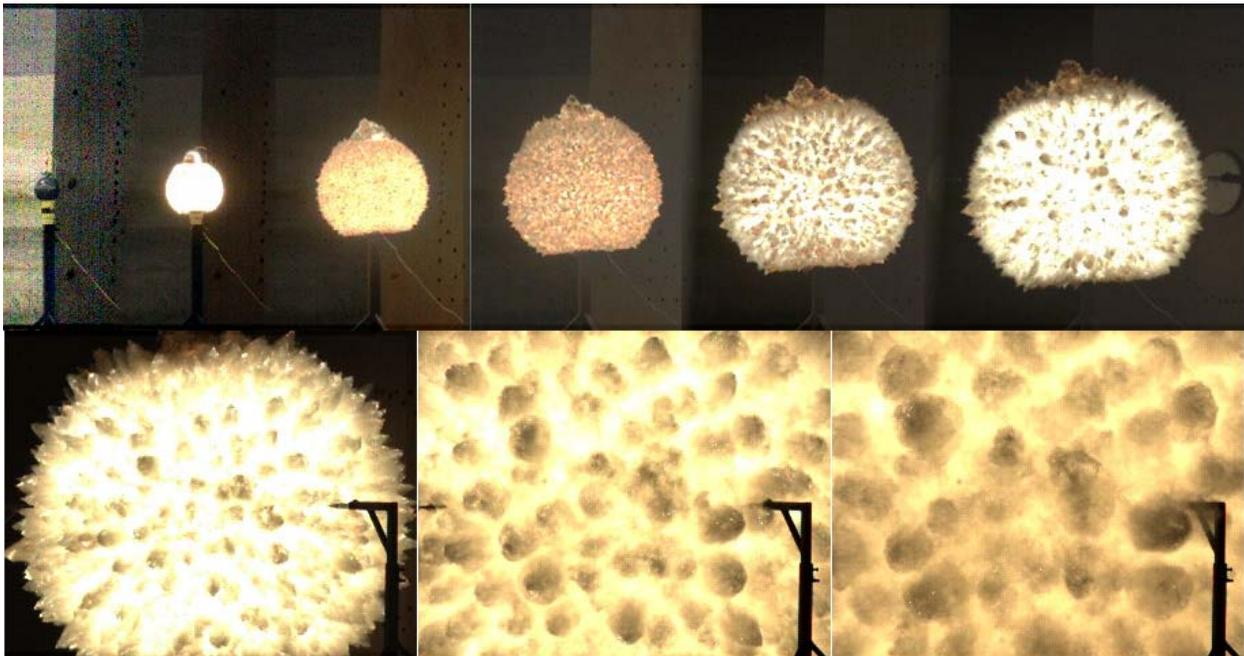
Fig. 2 Development of instabilities on fireball surface from detonation of 1 liter charge containing a packed bed of 600 – 850  $\mu\text{m}$  zirconium particles saturated with NM. Times for the photographs are 0, 40, 80, 120, 160, 200, 400, 800 and 1,200  $\mu\text{s}$ , respectively.
