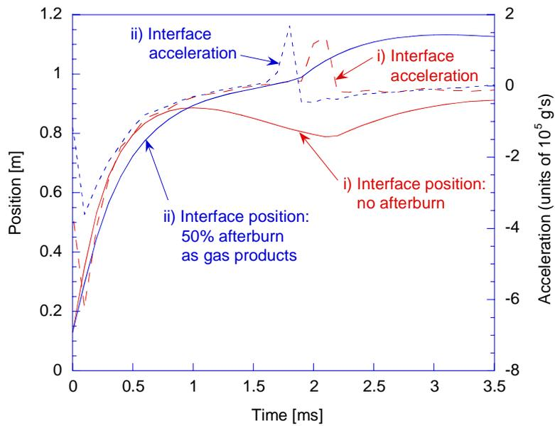
Fig. 4 Effect of afterburning on the motion of the combustion products interface. In case i) the energy is released instantaneously (no afterburn), whereas for case ii) 50% of the energy is released as afterburn.
