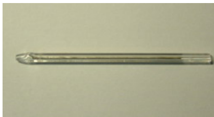
Fig 3: (a) Catalyst chamber, D=1\text{mm} and L=50\text{mm} (b) The ignition of decomposition reaction at 95% HTP flow rate 0.6\text{ cc / min} , the auxiliary power is 11\text{W} and exit temperature 978\text{ K} .
