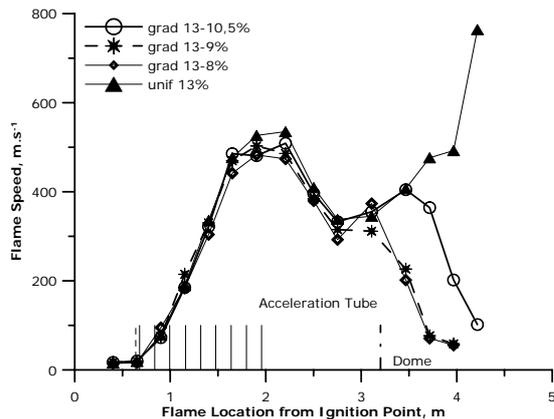
**Figure 3.** Flame speed vs. flame location in different negative  $H_2$  gradients in the tube (9 ring obstacles, bottom ignition)
