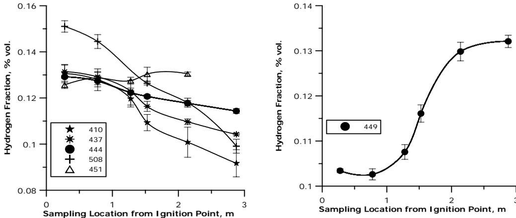
**Figure 1.** H<sub>2</sub> molar fraction according to distance from ignition point. Run# see table 1.
