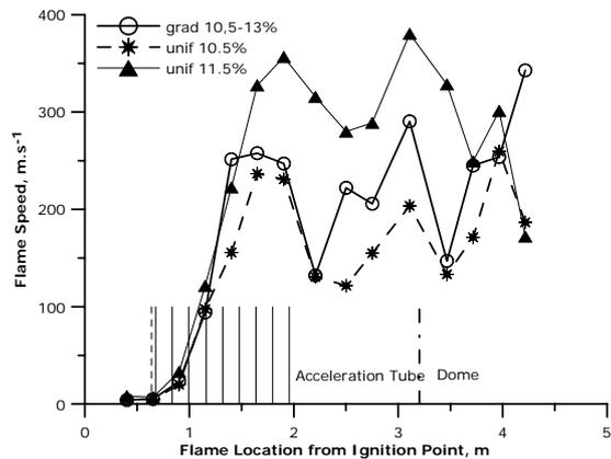
**Figure 4.** Flame speed vs. flame location in different positive  $H_2$  gradients in the tube (9 ring obstacles, bottom ignition)
