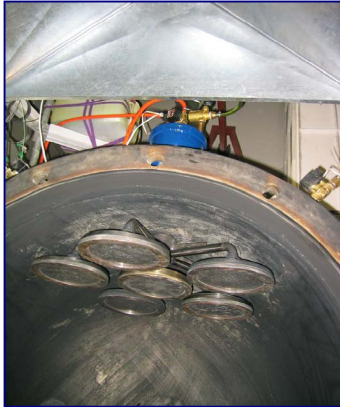
Fig.2. The view of the dispersing heads configuration inside the explosion chamber of 1,25m 3 volume.
