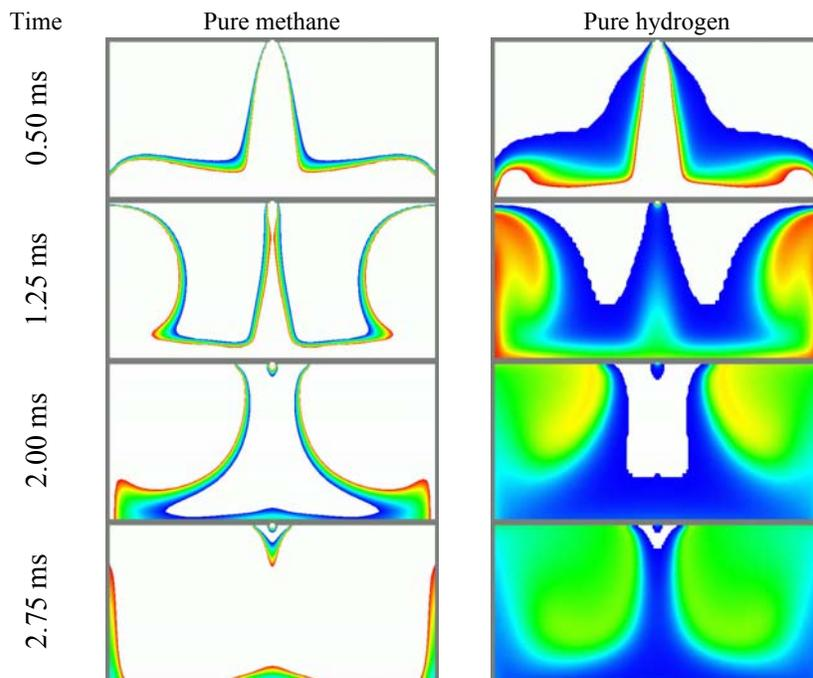
Fig.5. Flammable mixture zone for gaseous fuel injection to constant volume chamber.
