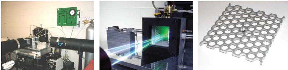
Fig. 1. Experimental set-up. (a) The view of entire system. Combustion chamber is located in the center. The Schlieren apparatus is to the front and right of the chamber. (b) Close-up view of the combustion chamber and LDA laser beams. The turbulence generating plates are shown inside. (c) Perforated plate for turbulence generation. The diameter of holes shown here is 10 mm.
