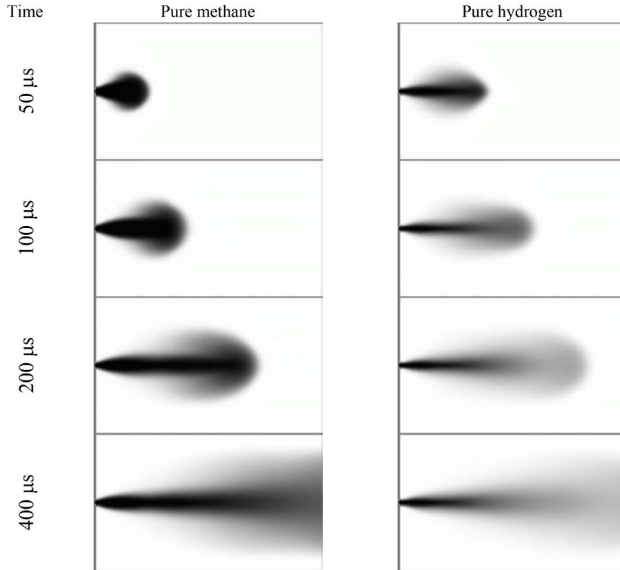
*Fig.3 Gaseous fuel jet structure for continuous injection to open space*
