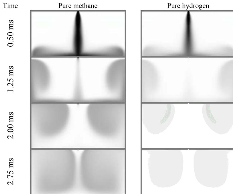
Fig.4. Gaseous fuel jet structure for injection to constant volume chamber
