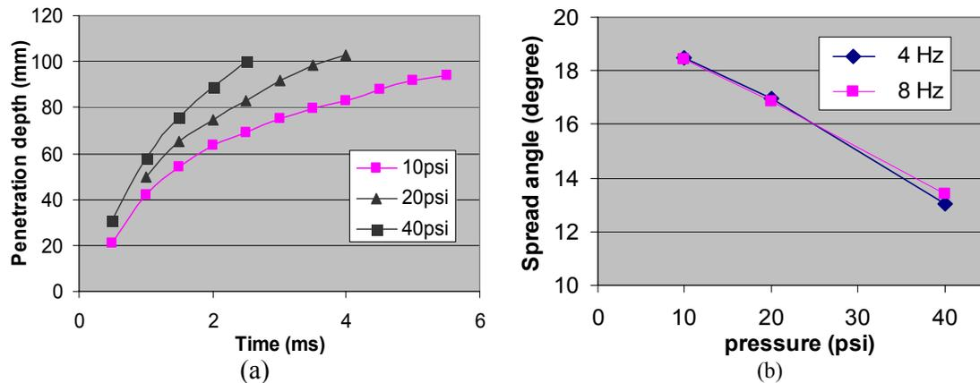
Fig. 2. Effect of injection pressure on penetration depth (a) and spread angle (b). Methane at 10, 20, 40 psi injected into chamber air;  $D = 3\text{mm}$ ;  $f = 8\text{ Hz}$  in (a) and 4 and 8 Hz in (b).
