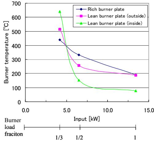
Fig. 8 Temperature of burner plates under the condition with all burners working
