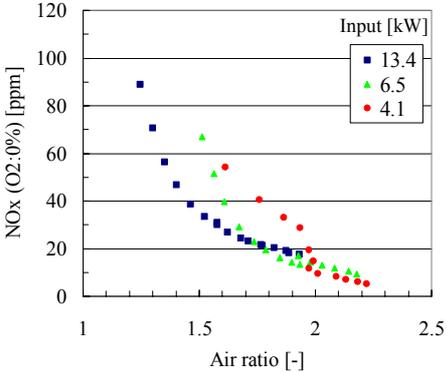
Fig. 6 NO<sub>x</sub> emission under the condition with all burners working
