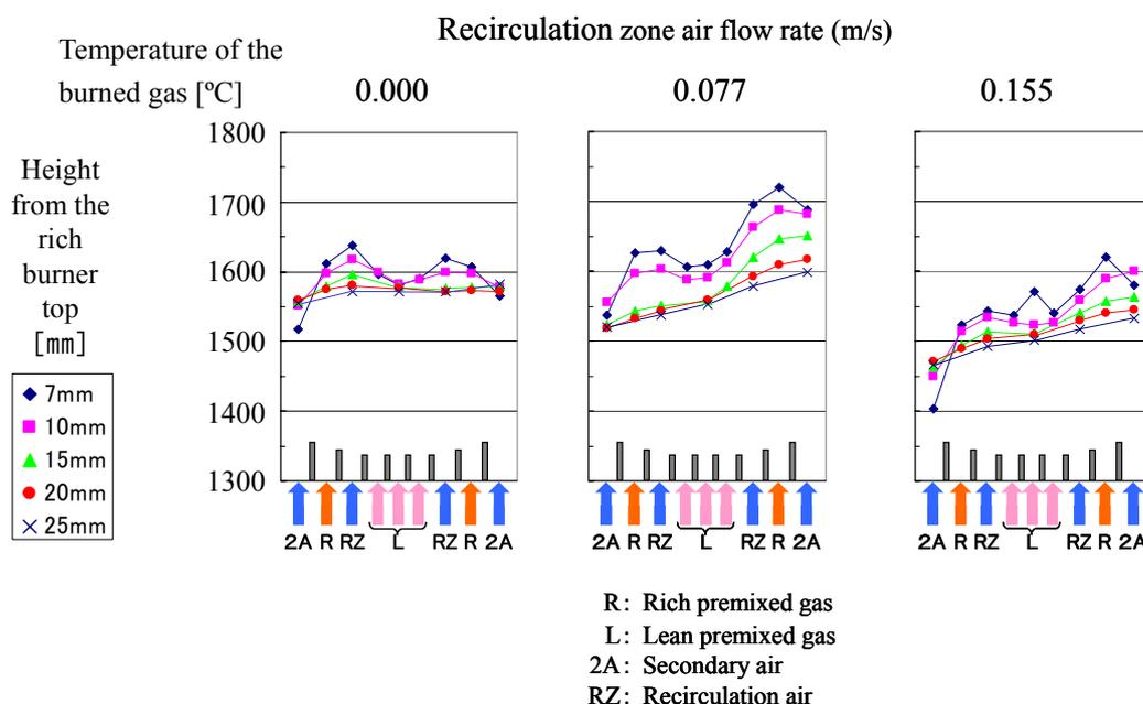
Fig. 12 Effect of air flow rate of recirculation zone on temperatures of burned gas
