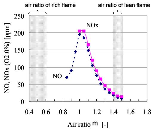
Fig. 2 NO<sub>x</sub> emission of premixed combustion at various air ratio  $m$
