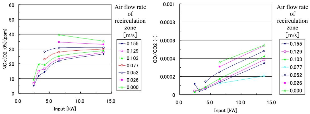
Fig. 11 Effect of the air flow rate of recirculation zone on the concentration of NO<sub>x</sub> and CO/CO<sub>2</sub>
