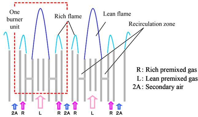
Fig. 1 Schematic figure of the conventional rich-lean flame burner
