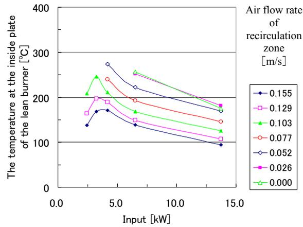
Fig. 10 The temperature of inside of lean burner plate
