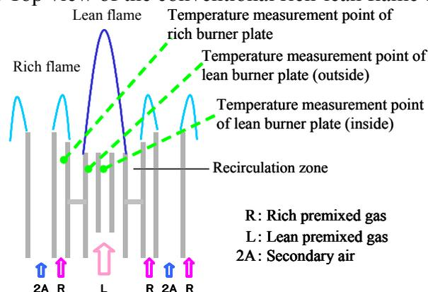
Fig. 5 Schematic figure of the points of measuring temperature
