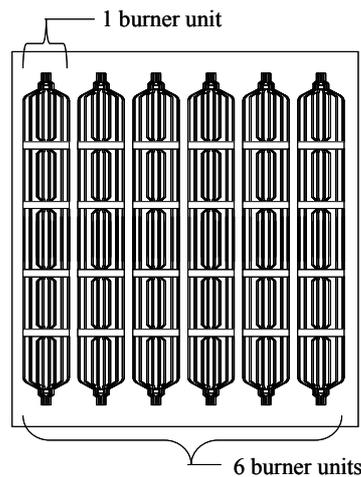
Fig. 4 Top view of the conventional rich-lean flame burner
