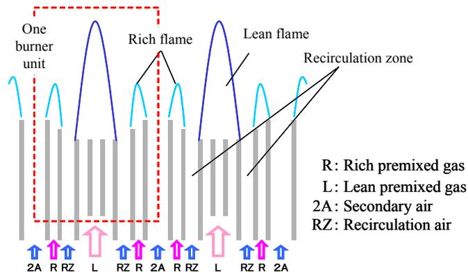
Fig. 9 Schematic figure of new type of rich-lean flame burner
