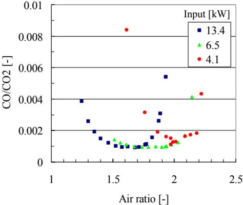
Fig. 7 CO/CO<sub>2</sub> under the condition with all burners working
