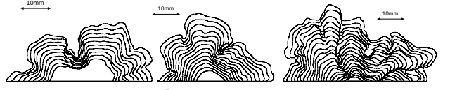
(a)M08-25NH00(b)M08-25NH05(c) M08-25NH10 Fig. 2 Temporal Evolution of Flame Front Contours ( u'/S_{L0} \approx 1.4 )
