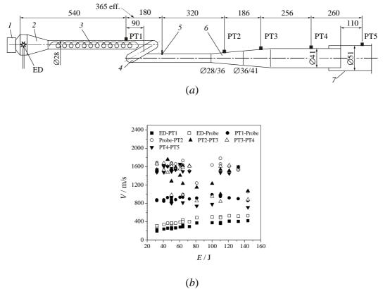
Fig. 2 (a) Schematic of 28-millimeter tube with tube coil and conical transition sections to the main tube 51 mm in diameter. (b) Measured shock wave velocities in a two-phase n-hexane-air mixture at different measuring segments as a function of ignition energy
