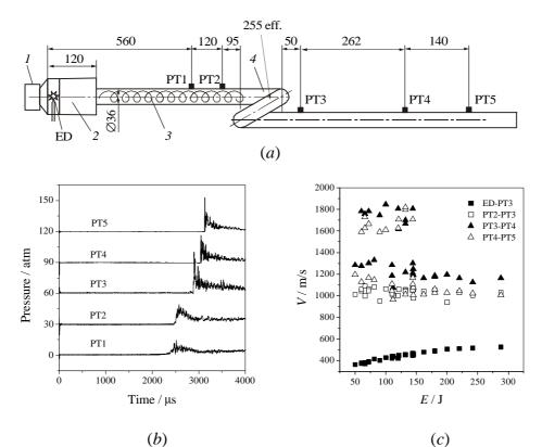
Fig. 1 (a) Schematic of 36-millimeter tube with a new element — tube coil. (b) Pressure records by gauges PT1, PT2, ..., PT5 in the run with ignition energy of 60 J. (c) Measured shock wave velocities in a two-phase n-hexane—air mixture at different measuring segments as a function of the ignition energy
