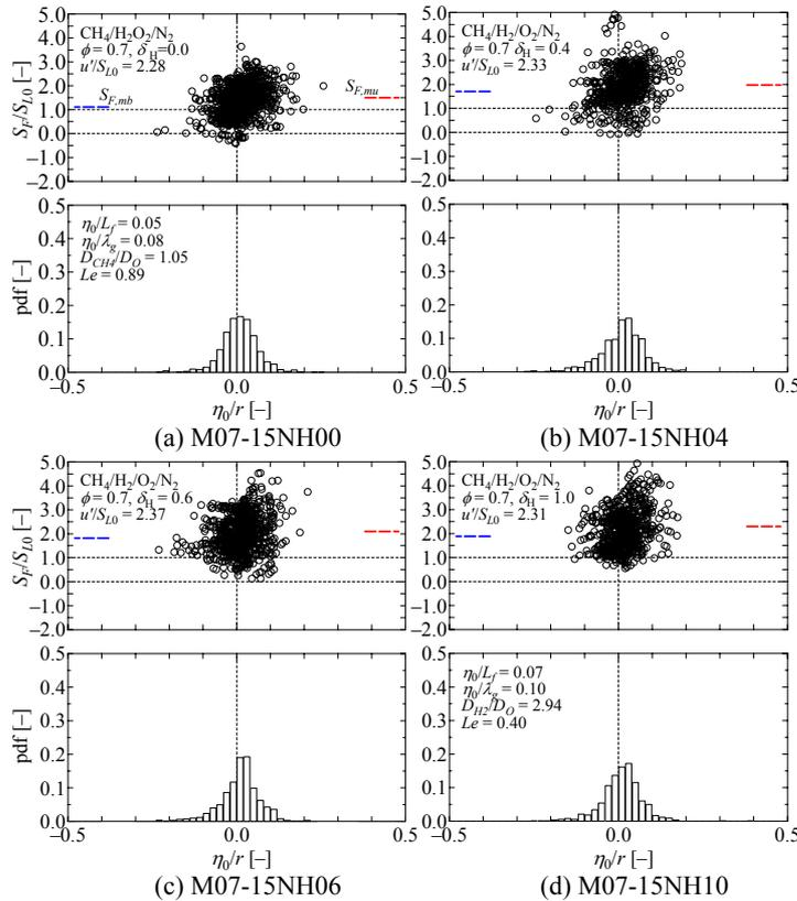
Fig.4 Pdf of the curvature and distribution of the local flame displacement velocity ( $u'/S_{L0} \approx 2.3$ ,  $(R_A/R_C)^3 \approx 0.018$ )
