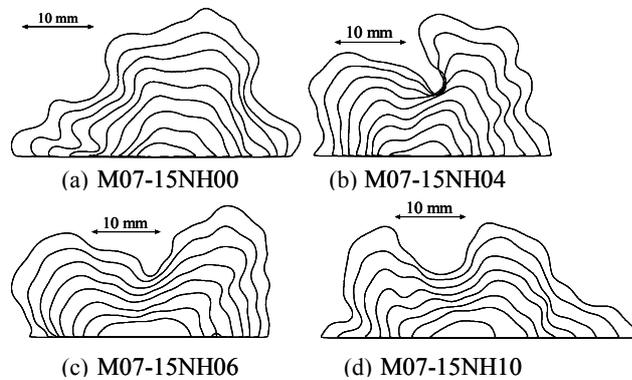
Fig.3 Temporal evolution of flame-front contours (every 1ms,  $u'/S_{L0} \approx 2.3$ )
