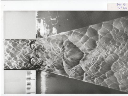
Figure 4. Soot-plate record demonstrating detonation transition at  $P_o=0.04$  bar and  $\alpha=15^\circ$ .
