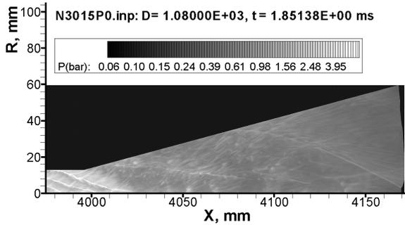
Figure 8. Calculated traces of maximum pressure at  $P_o=0.03$  bar and divergence angle  $\alpha=15^\circ$  ( $t=1.851$  ms).
