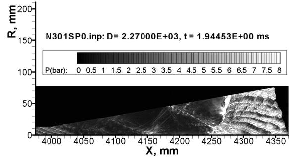
Figure 9. Calculated traces of maximum pressure at  $P_o=0.03$  bar and  $\alpha=10^\circ$  ( $t=1.944$  ms).
