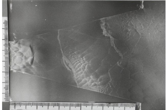
Figure 3. Soot-plate record after detonation transition at  $P_o=0.035$  bar and divergence angle  $\alpha=15^\circ$ .
