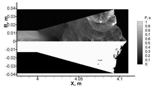
Figure 11a. Distributions of scaled pressure,  $P/(2 \text{ bar})$ , (at  $R>0$ ) and reaction product concentration  $a$  (at  $R<0$ ) at  $P_o=0.04$  bar,  $\alpha=15^\circ$ ,  $t=1.769$  ms.
