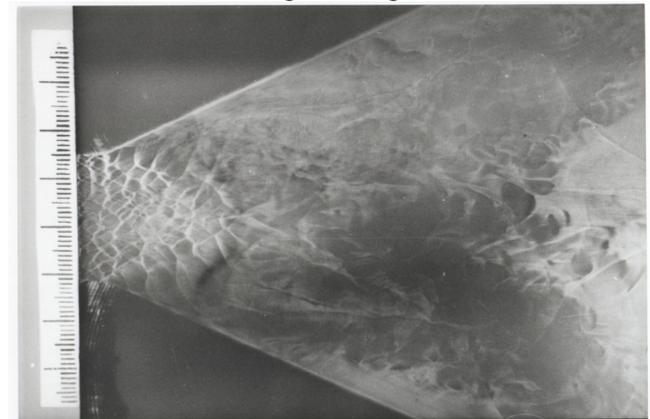
Figure 5. Soot-plate record showing detonation extinction at  $P_o=0.04$  bar but higher  $\alpha=25^\circ$ .
