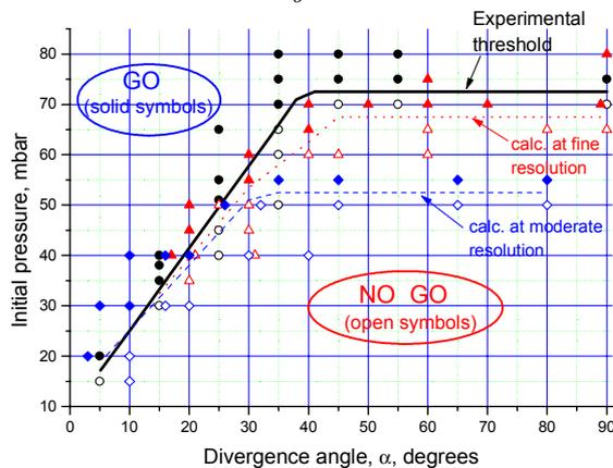
Figure 6. Dependence of critical pressure on divergence angle for 26-mm diameter tube. Triangles and diamonds show numerical results.
