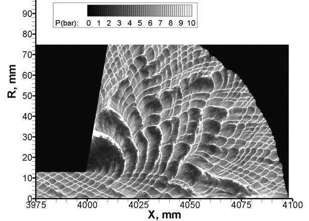
Figure 12. Transition at  $P_o=0.07$  bar and divergence angle  $70^\circ$  ( $t=1.729$  ms)
