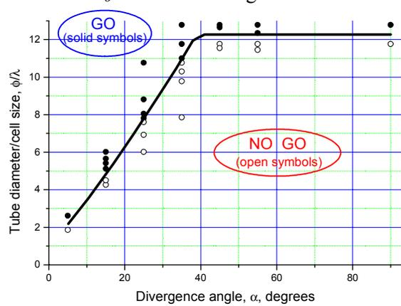
Figure 7. Dependence of ratio of tube diameter to critical detonation cell size for both 26- and 52-mm diameter tubes.
