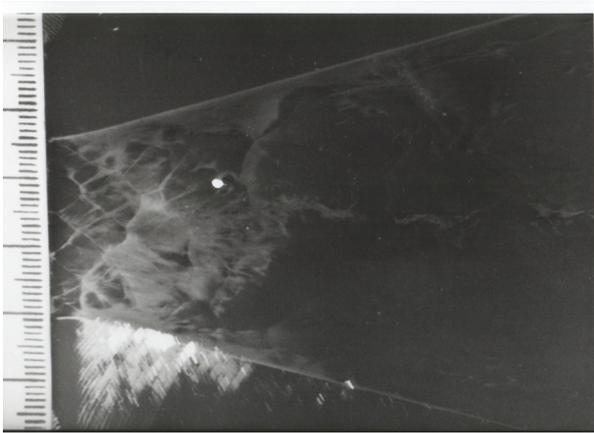
Figure 2. Soot-plate record after detonation extinction at  $P_o=0.03$  bar and  $\alpha=15^\circ$ .
