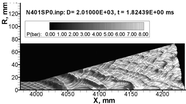
Figure 10. Transition at  $P_o=0.04$  bar and divergence angle  $15^\circ$  ( $t=1.824$  ms).
