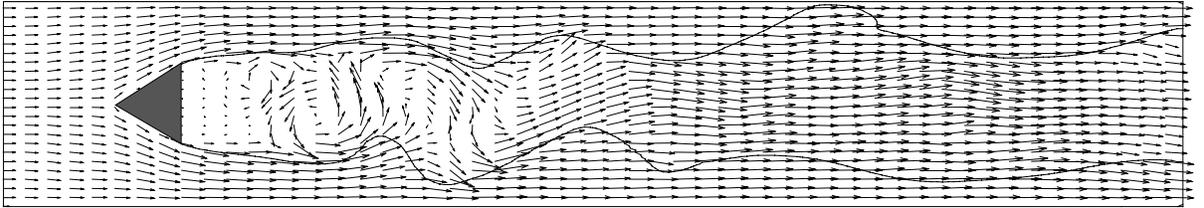
**Figure 1.** An instantaneous flame front ( $G=0$ ) and velocity vectors plotted on a course grid (one fourth of grid points in each direction is shown).
