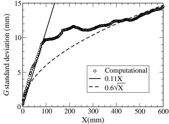
**Figure 4.** Time averaged standard deviation of  $G, \sqrt{G^2}$ , at the flame front ( $\bar{G} = 0$ ) along axial direction.
