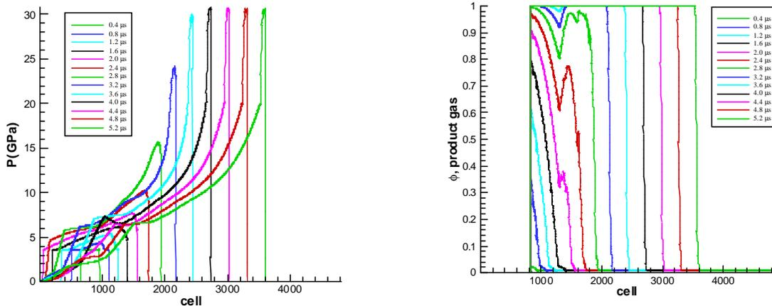
Fig. 1. Growth-to-detonation behavior is shown in (a) where the steady detonation propagates at the velocity of 8 km/s. The value in a LASL report is 8.6 km/s at 33.7 GPa (CJ state). Fractions of the product gas shown in (b) indicate an heterogeneous ignition.
