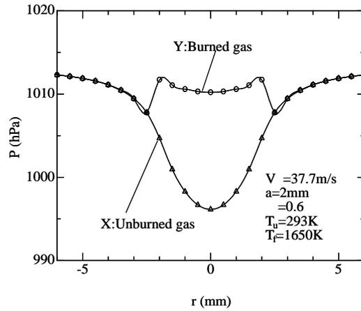
Figure 6 Pressure distributions of the unburned and burned gases
