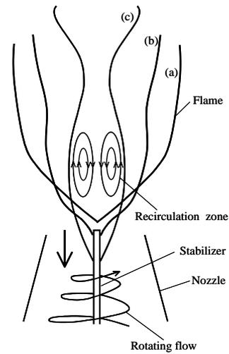
Figure 8 Stabilization mechanisms of the inverted flames established in the rotating flow
