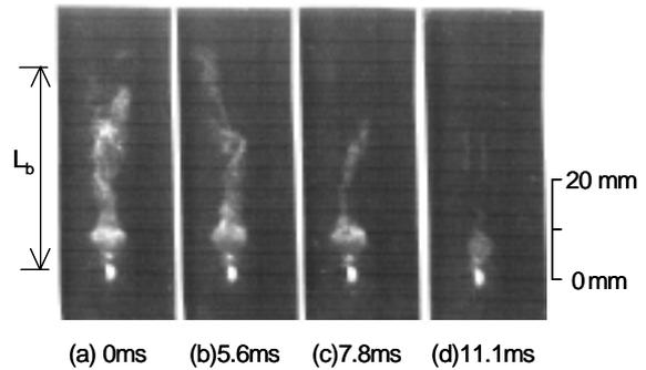
Figure 4 Flames at an instant of blow-off
