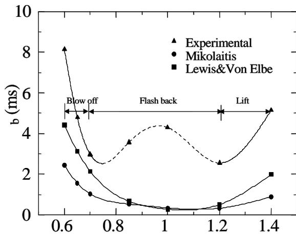
Figure 7 Characteristic ignition times at stability limits
