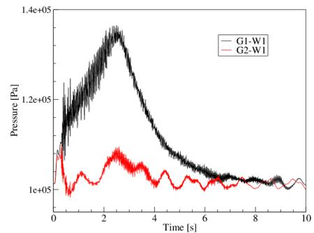
Figure 4: Pressure time history at nozzle for two geometries G1 and G2
