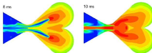
Figure 5: Temperature contour plots for methane-air combustion at 8 and 10ms. Geometry G1 and ignition configuration W1 (ignition only on back wall).
