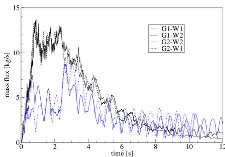
Figure 3: Mass flow time history at nozzle for ignition arrangements W1 and W2 comparing two geometries G1 and G2
