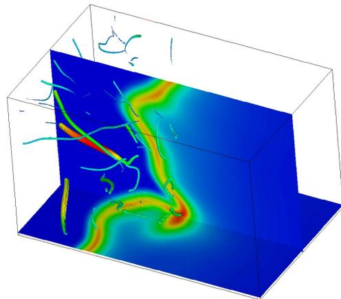
Fig. 7 Distributions of heat release rate and the axes of fine scale eddies for Case 1.
