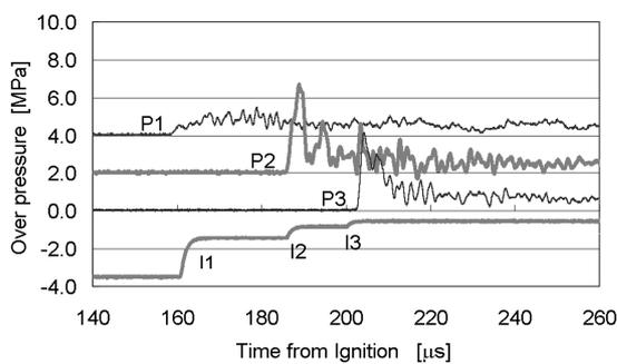
Fig3 Propagation of shock wave (pressure transducer) and flame (ion probe) in  $H_2-O_2$  initiator.
