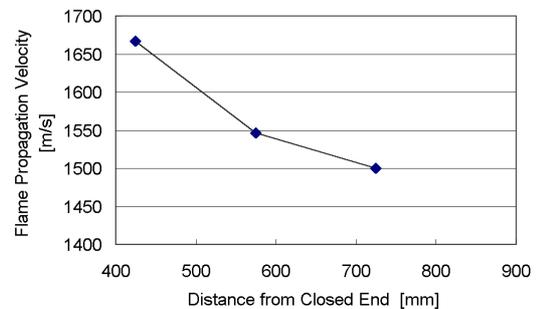
Fig8 Flame propagation velocity in the main tube partially filled with gasoline-air mixture, using gasoline- $O_2$  initiator.
