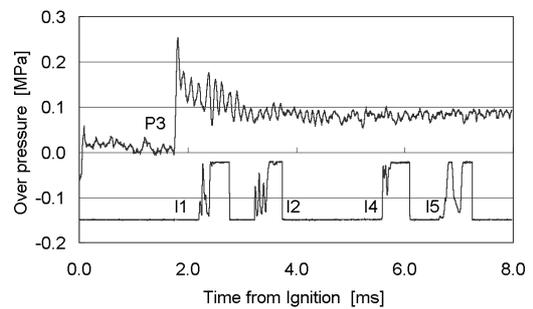
Fig4 Propagation of shock wave (pressure transducer) and flame (ion probe) in gasoline-air mixture in main tube, using  $H_2-O_2$  initiator.
