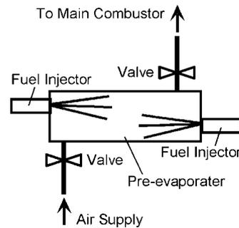
Fig6 Schematic diagram of pre-evaporator
