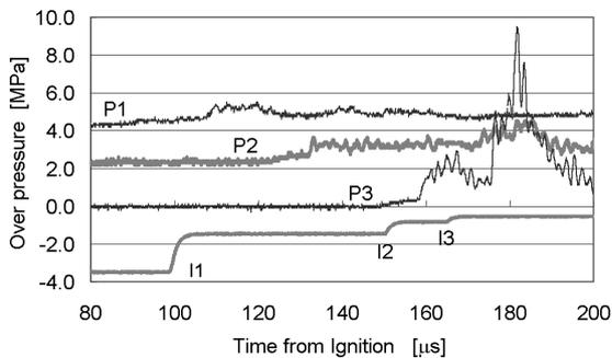
Fig5 Propagation of shock wave (pressure transducer) and flame (ion probe) in gasoline- $O_2$  initiator.
