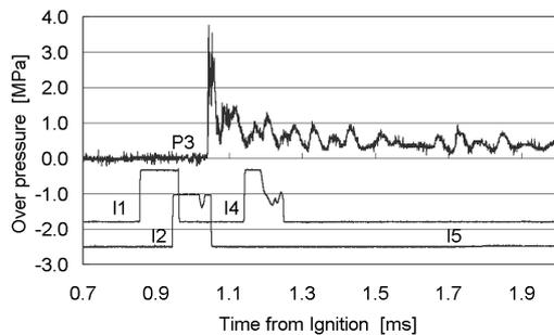
Fig7 Propagation of shock wave (pressure transducer) and flame (ion probe) in gasoline-air mixture in main tube, using gasoline- $O_2$  initiator and pre-evaporator.
