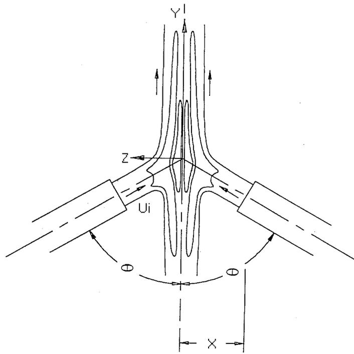
Figure 1: Configuration of jet-to-jet impingement
