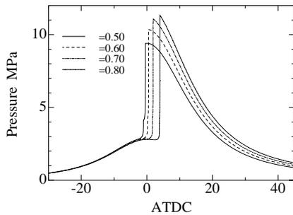
Fig. 4 Pressure history ( $\phi = 12.0$ ,  $T_{\text{ini}} = 295\text{K}$ ,  $\phi = 0.50 \sim 0.80$ )
