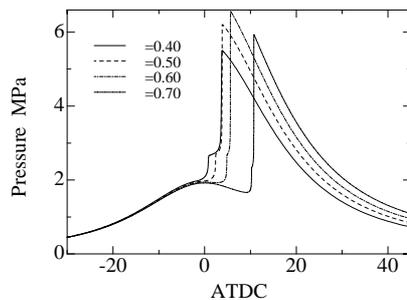
Fig. 1 Pressure history (  $\phi=9.0$ ,  $T_{ini}=320K$ ,  $\phi=0.40 \sim 0.70$  )
