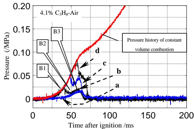
Fig.5. Pressure history for at different venting pressures and for vent diameter 100mm (venting pressure in MPa: a—0.005 ; b—0.02 ; c—0.05 ; d—0.08).
