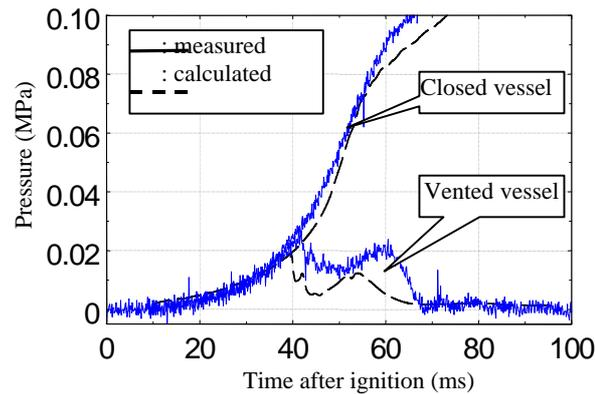
Fig.8. Comparison of measured and calculated pressure-time curves both in closed and vented vessels.
