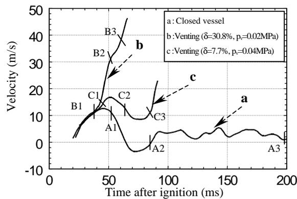
Fig.3. Comparison of flame propagation velocities for closed and venting vessels. A, B, C indicate characteristic points on velocity curves.
