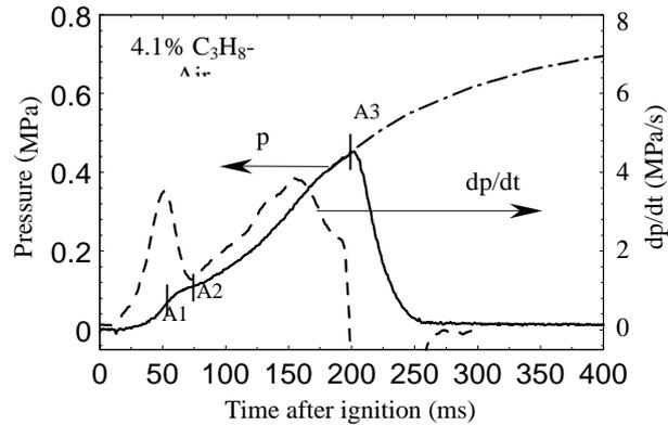
Fig.4. Pressure history and rate of pressure rise in constant volume explosion.
