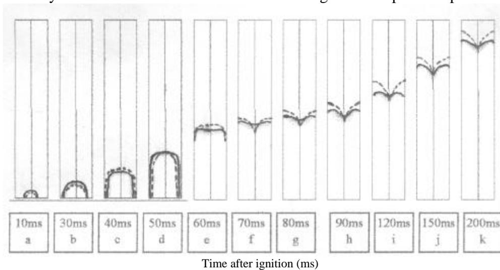
Fig.7. Comparison of calculated and measured results of flame front evolution in closed vessel. Calculated – continuous line. Measured – dashed line.
