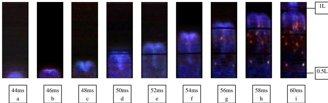
Fig.6. Flame propagation during venting with vent diameter 100mm and mixture concentration 4.1%  $C_3H_8$   $P_v=0.02MPa$ ,  $t_v=42ms$ ,  $\delta=30.8\%$ .
