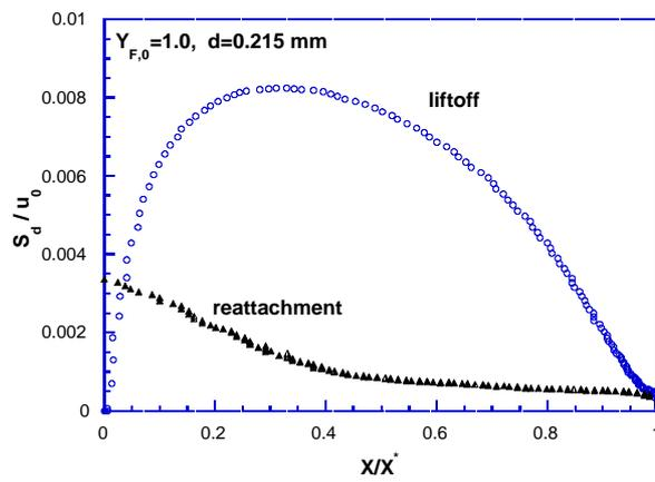
Figure 5 Transient displacement speeds during liftoff and reattachment.
