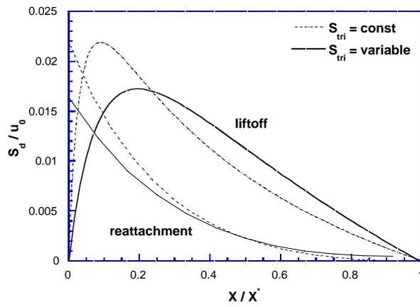
Figure 4 Calculated transient displacement speeds during liftoff and reattachment.
