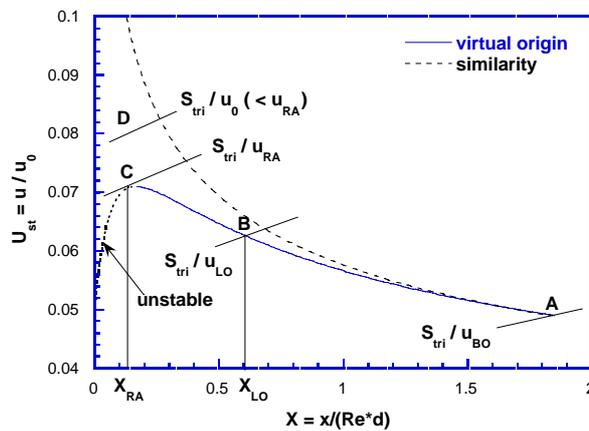
Figure 2 Calculated axial velocity profile along stoichiometric contour for propane jet.
