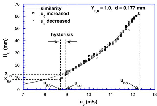
Figure 1 Comparison of liftoff height between experiment and similarity prediction with nozzle exit velocity.
