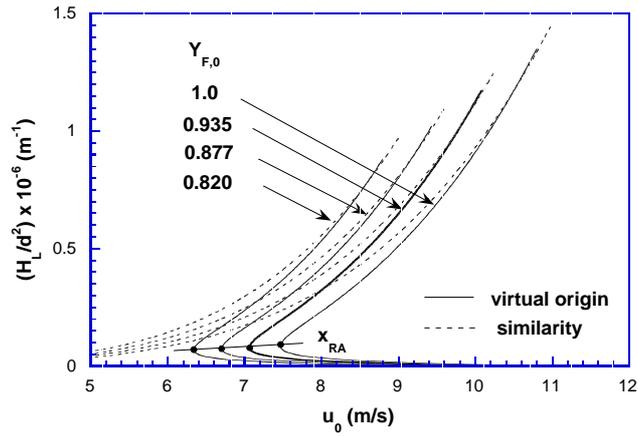
Figure 3 Calculated liftoff height with nozzle exit velocity.
