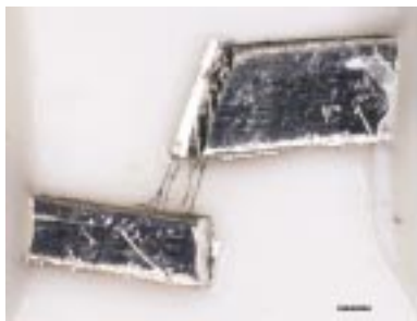
Figure 4. Growth of silver oxide filaments bridging electrode gap at low power.
