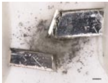
Figure 5. Mature silver oxide deposit, R < 100\Omega .
