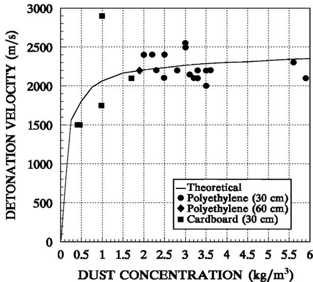
Figure 4. Detonation velocity versus dust concentration for RDX-air mixtures.
