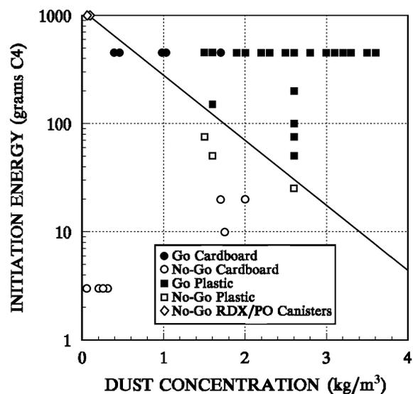
Figure 6. Initiation energy versus dust concentration for RDX-air mixtures.
