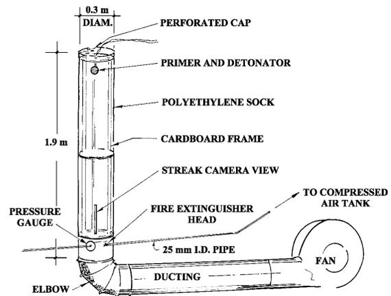
Figure 3. Pictorial of vertical detonation tube used in the RDX dust detonation studies.
