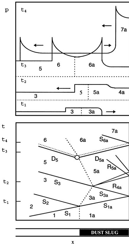
Figure 7. Wave diagram for DDT in an end multiphase slug.
