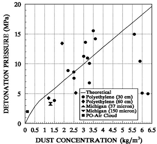
Figure 5. Detonation pressure versus dust concentration for RDX-air mixtures.
