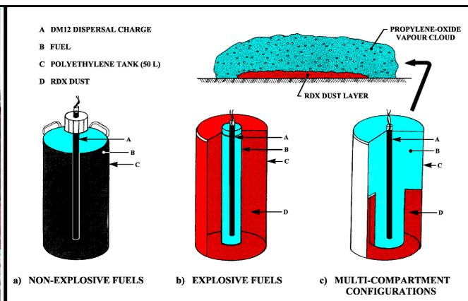
Figure 2. Canister configurations for: (a) non-explosive fuels, (b) high-explosive fuels, and (c) hybrid fuels.
