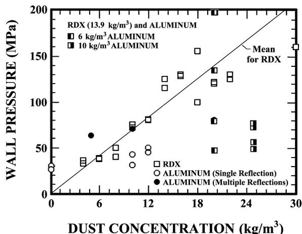
Figure 8. Peak wall pressure versus dust concentration in 6.75% acetylene-air with a 100-mm end slug of RDX or aluminum dust.
