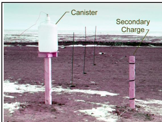
Figure 1. Photograph of typical canister and secondary charge used in detonation experiments.
