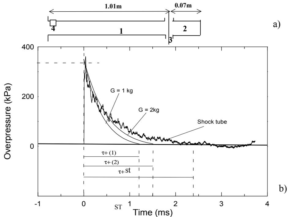
**Fig. 1** Pressure histories recorded in a shock tube in comparison with HE explosion.
