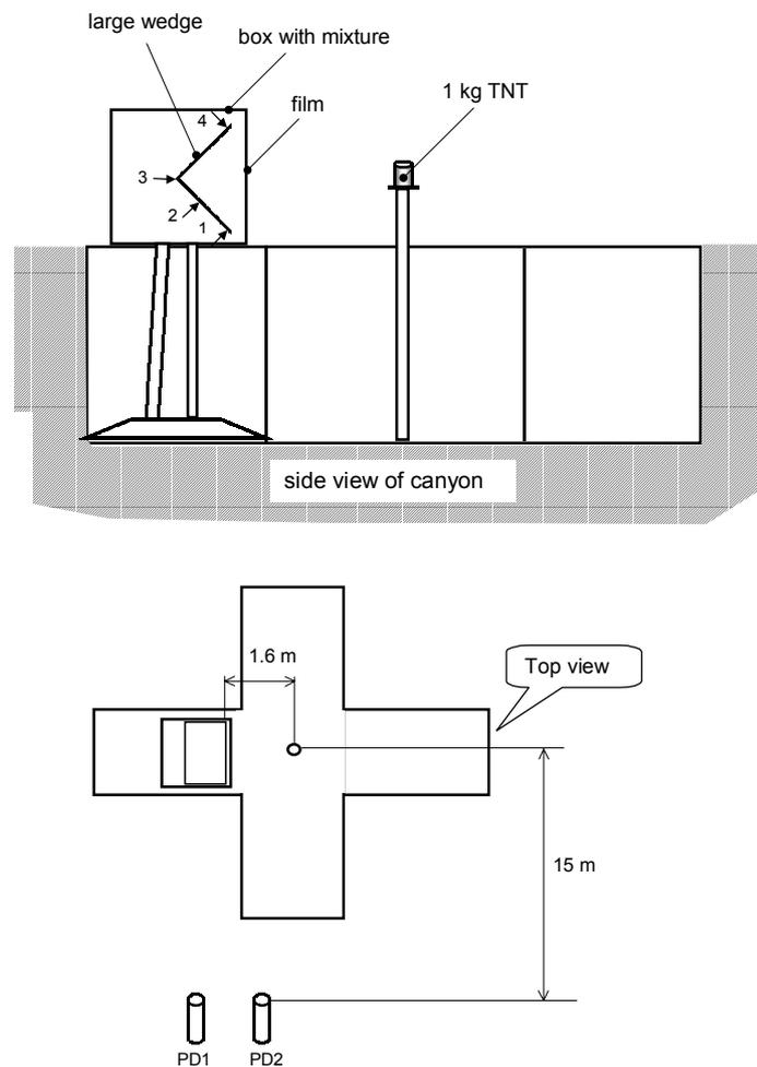
**Fig.2** Scheme of the experimental facility for study of hydrogen-air combustion under conditions of blast.
