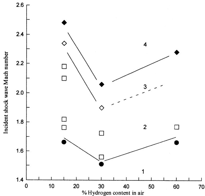
**Fig.3** Areas of explosive modes for wedge reflector with a corner  $90^0$ .
