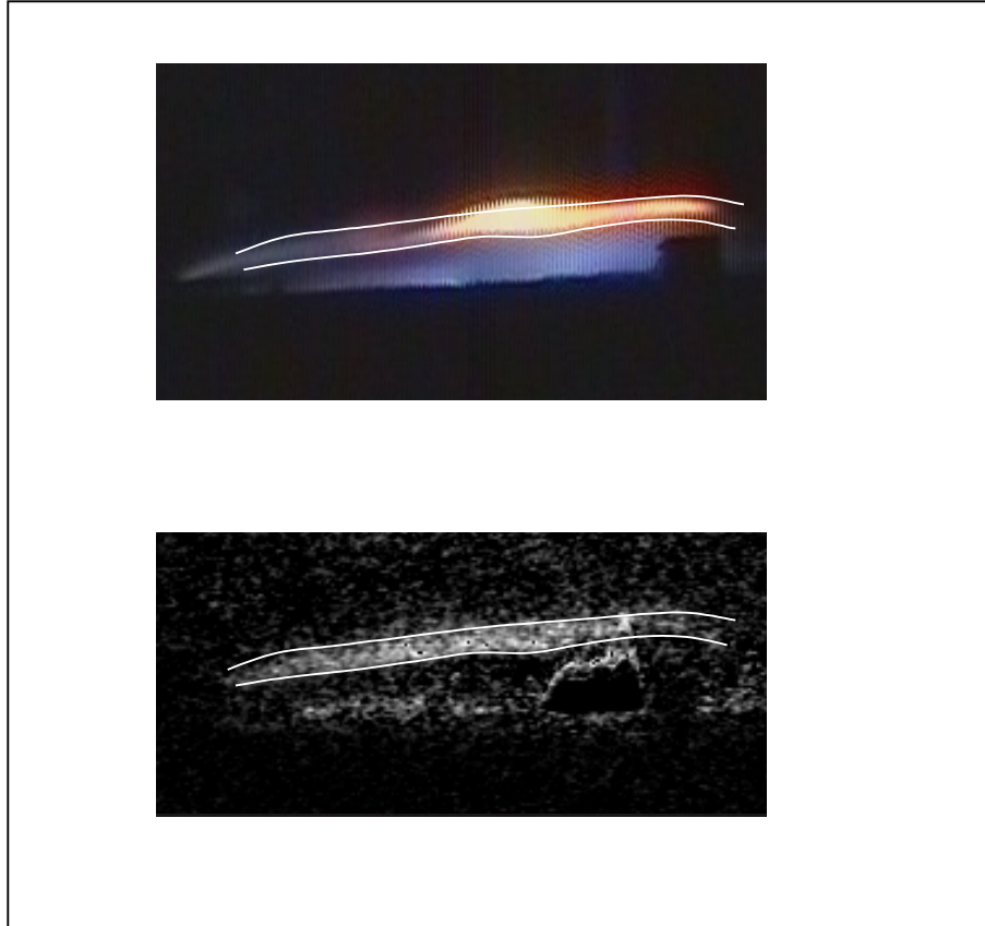
Figure 1 : Comparison between OH (PLIF) and visible flame emission
