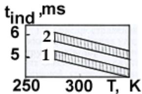
Figure 5. Pre-detonation time in air - gasoline mixtures: 1 - A-76; 2 - A-93.
