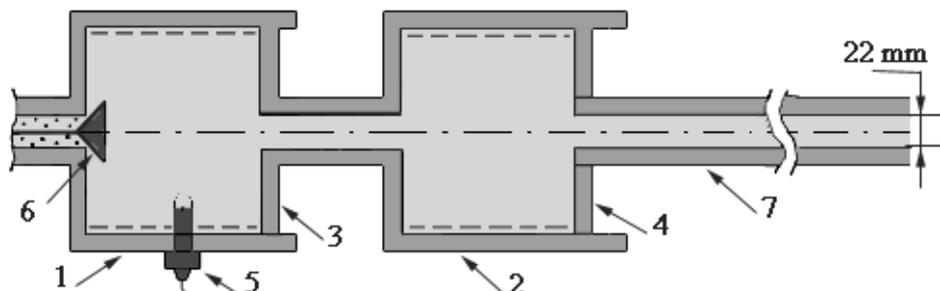
ignition sections of the tube (Fig. 1) promoted the onset of detonation by shortening essentially the pre-detonation length for hydrocarbon fuels – air mixtures.
