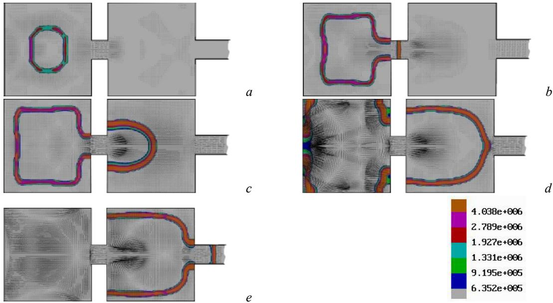
Figure 6. Chemical reaction zone evolution for successive times after ignition: *a*- 1ms, *b*- 3.1ms, *c*- 3.7ms, *d*- 4.2ms, *e*- 4.4ms.
