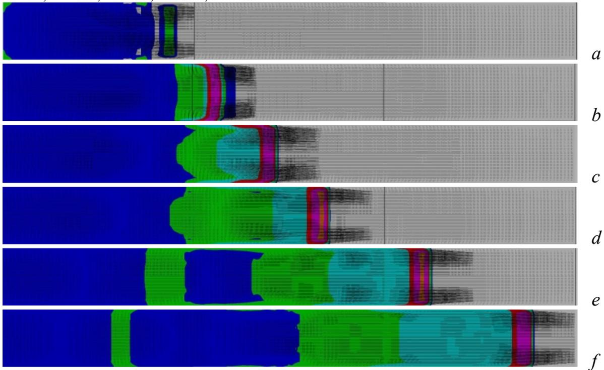
Fig.7. Pressure evolution in the detonation tube in the transition zone for successive times: *a*- 4.593 ms, *b*- 4.628 ms, *c*- 4.643 ms, *d*- 4.657 ms, *e*- 4.683 ms, *f*- 4.709 ms.
