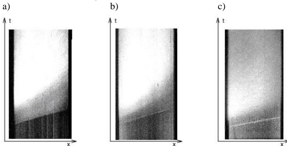
**Fig 2. Streak photographs of ignition of: a) kerosene, b) nitroglycerine, c) PNT**
