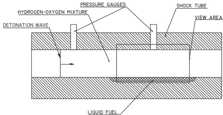
**Fig 1. Schematic diagram of visualisation section.**
