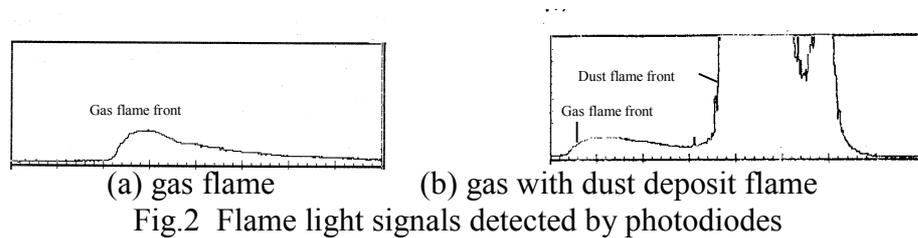
Fig.2 Flame light signals detected by photodiodes
