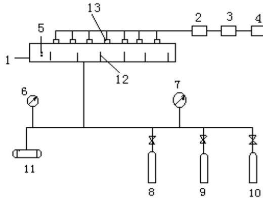
1.FAT 2.Electricity transducer 3. Data acquisition and digital transient recorder 4.Printer 5.Spark ignition source 6.Manometer 7.Vacuum-meter 8.Gas mixture 9.Air 10.Methane 11.Vacuum-pump 12.Obstacle 13. Photodiode
