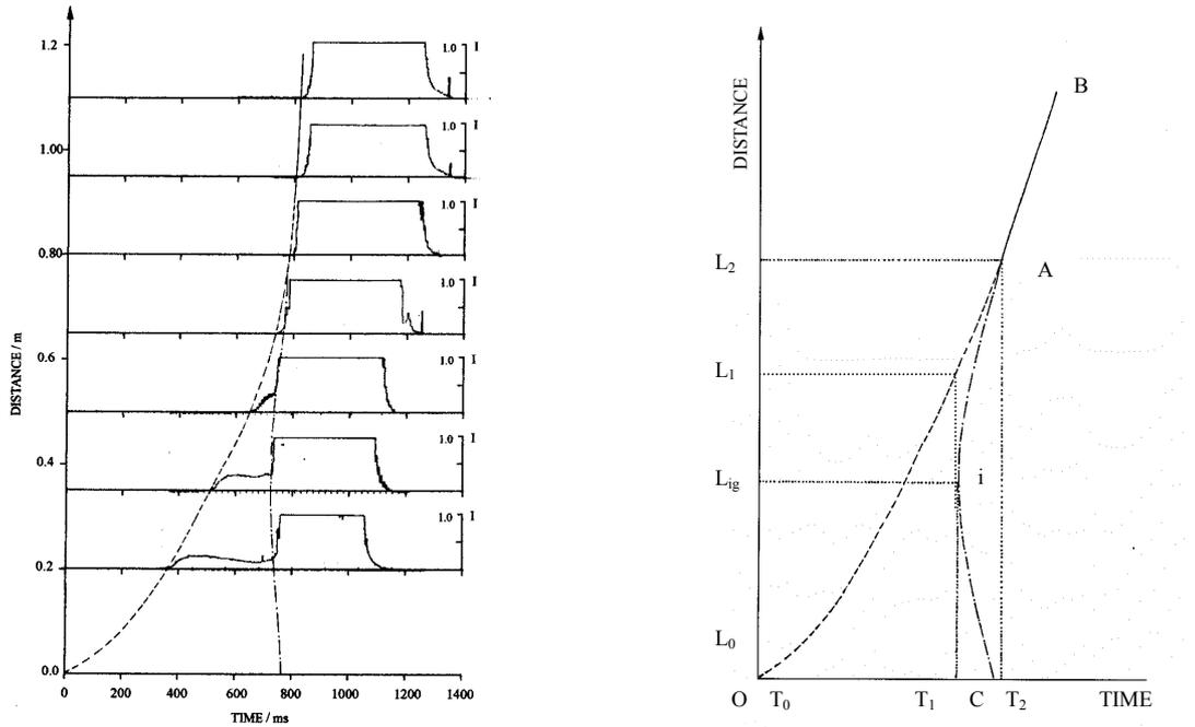
Fig.3 The trajectory of complicated gas-deposited dust flame
