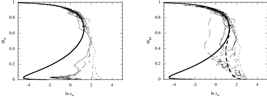
Figure 2: Temporal development of arbitrary extinguishing particles (thin lines). Thick lines are steady state solutions of Eq. (10) for  $\langle \Upsilon_{st} \rangle = 0$  (solid line) and  $\langle \Upsilon_{st} \rangle = 10$  (dashed line)
